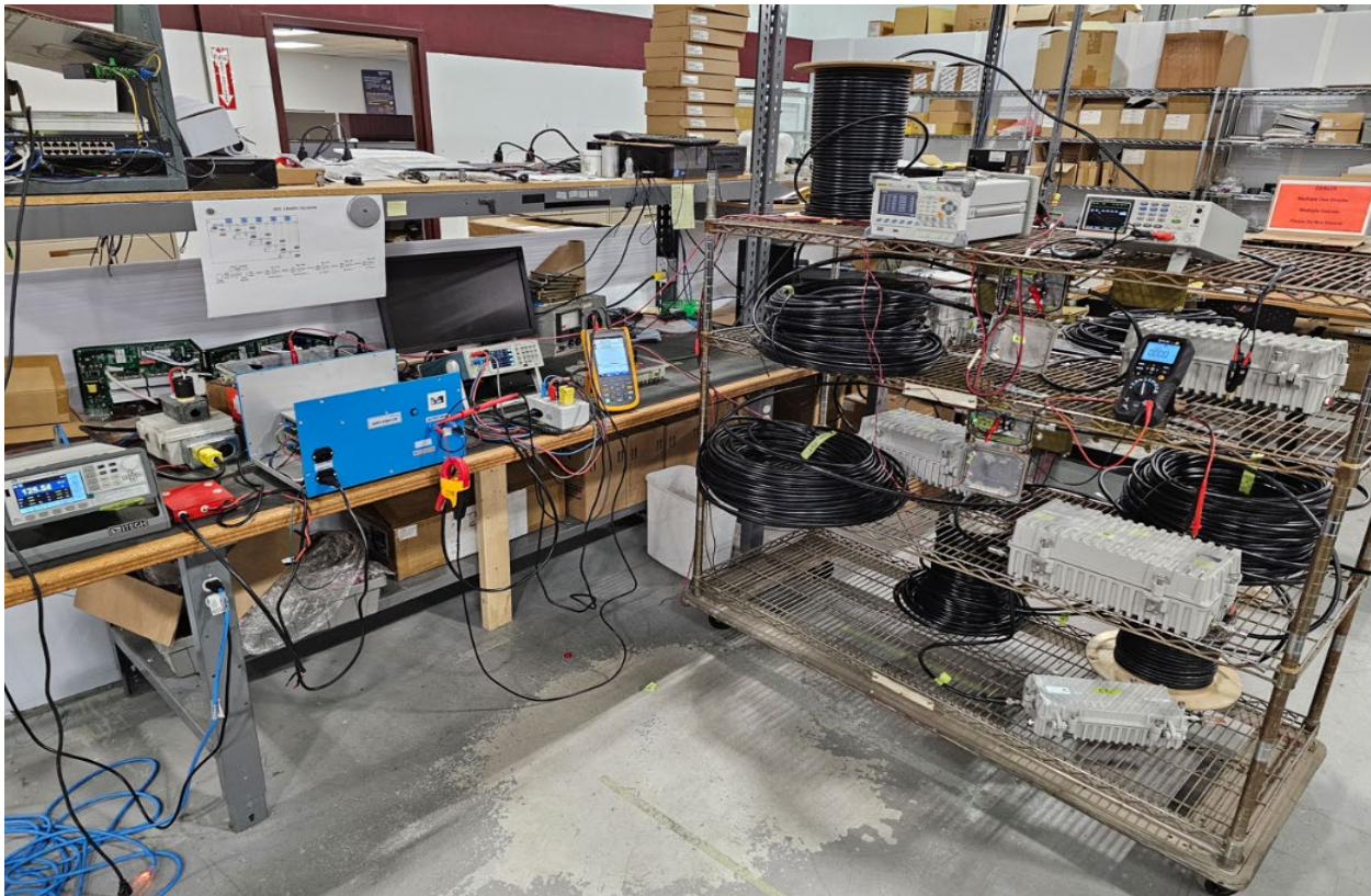
Figure 9 – 5-Amplifier Cascade Performance Testing Set-up - Picture
