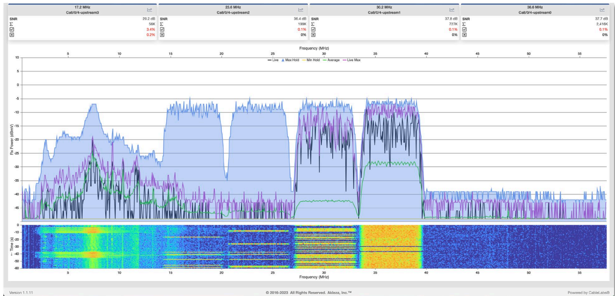
Figure 6 - Example UTSC Display Showing Ingress Noise
