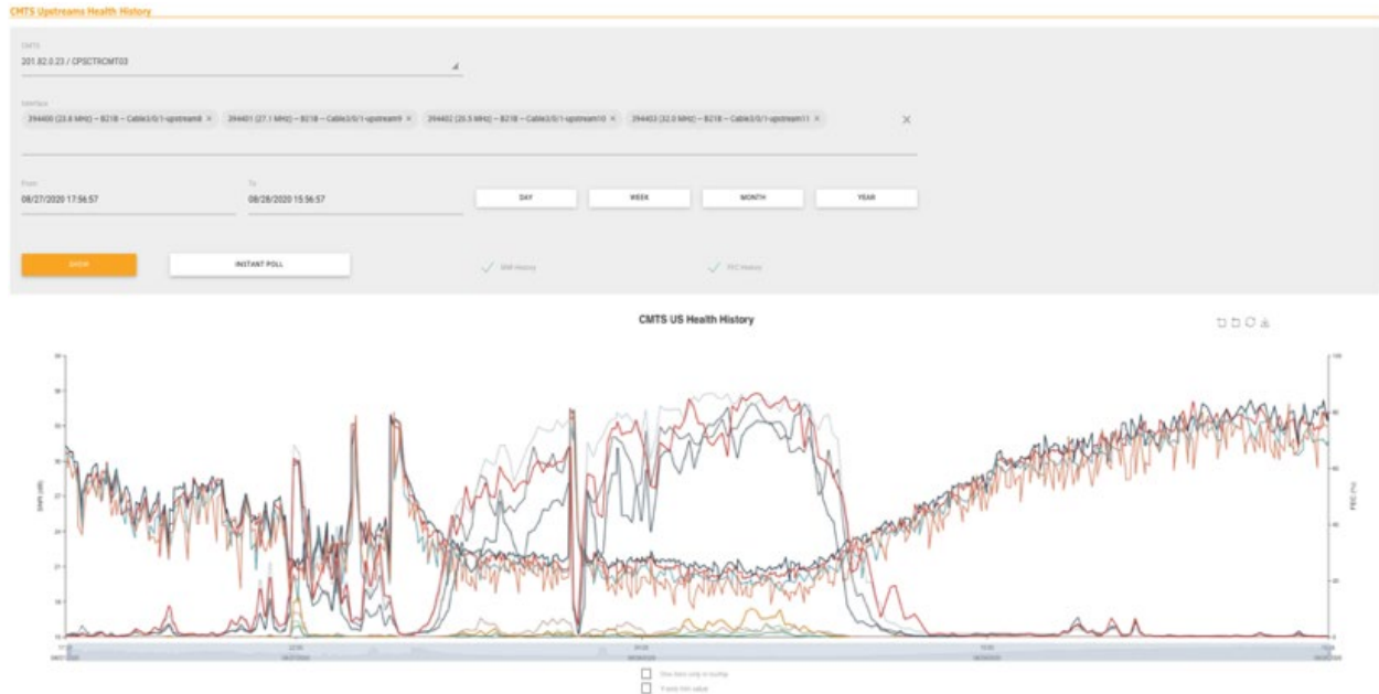
Figure 18 - Upstream SNR and Codeword Errors of upstream channels in a service group over time, showing a complex noise and impairment situation in the network
