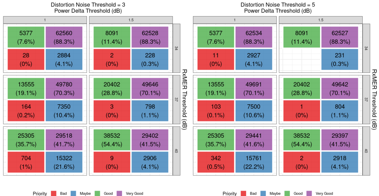
Figure 11 - Results of simulations exploring different High/Low thresholds for Distortion Noise, RxMER, and Power delta. The left panel is for distortion noise threshold of 3 dBmV and right panel a threshold of 5 dBmV. Within each panel the columns correspond to Power Delta threshold of 1 and 1.5 dB and the rows correspond to RxMER thresholds of 34, 37 and 40 dB. The outcome is the number and percent of RPDs placed in each of the priority groups.
