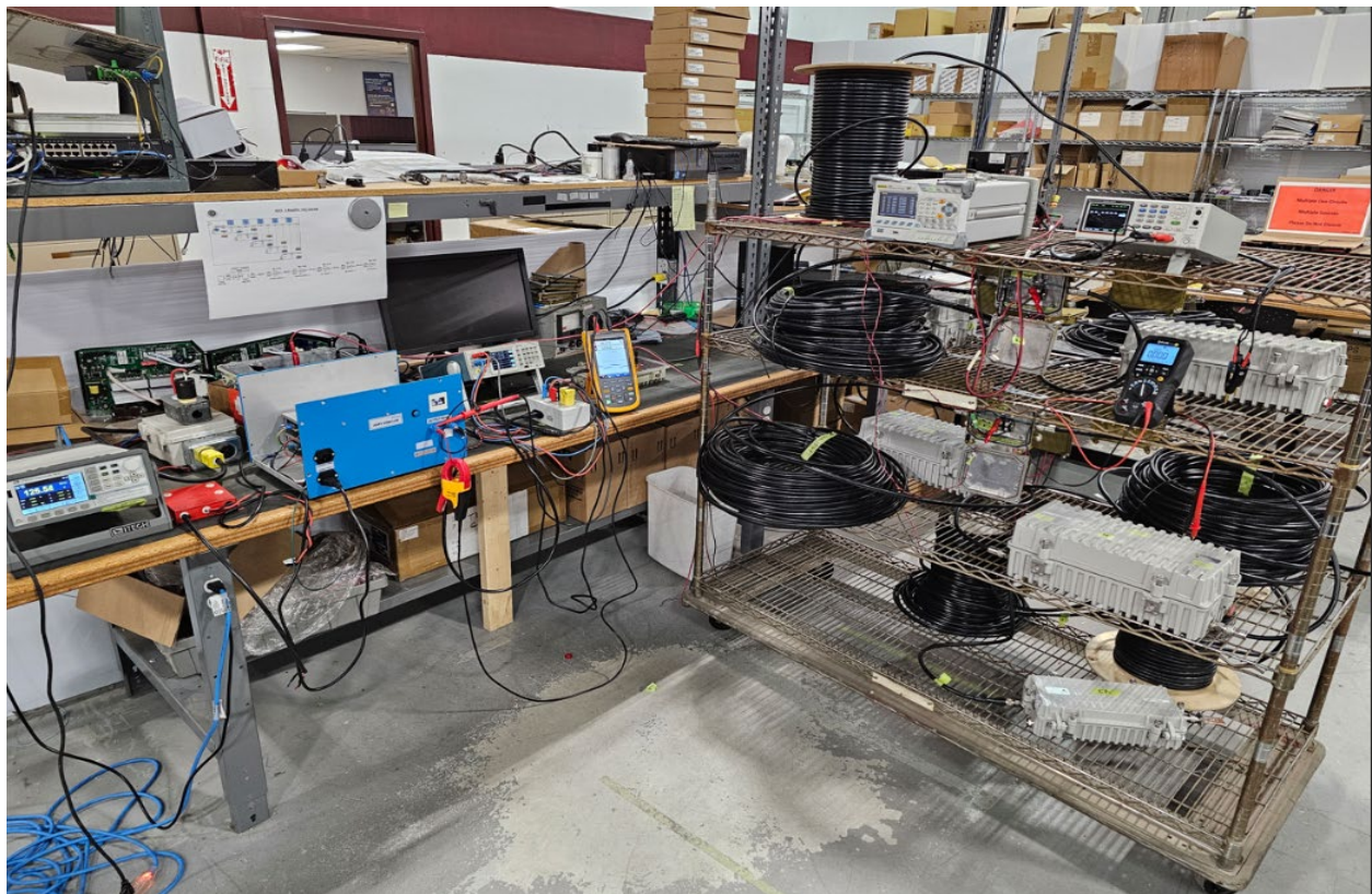
Figure 9 – 5-Amplifier Cascade Performance Testing Set-up - Picture
