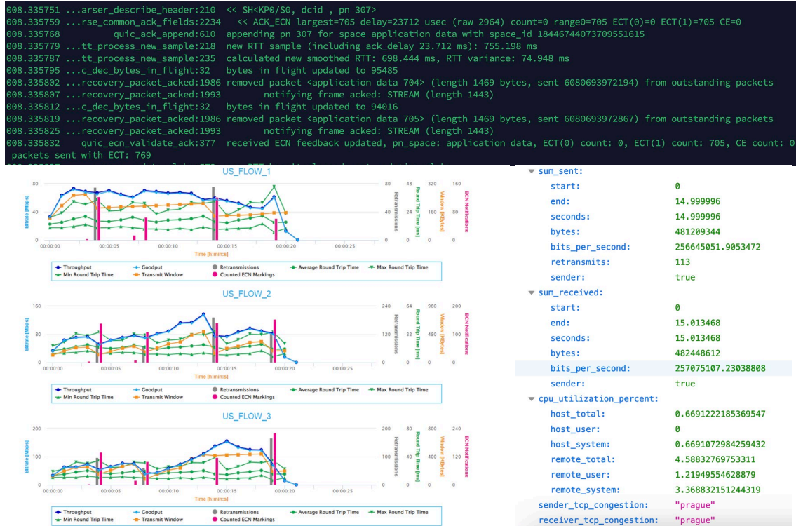
Figure 2 – L4S traffic models : Top: Apple L4S QUIC; Bottom Left: Excentis ByteBlower L4S; Bottom Right: Linux TCP Prague
