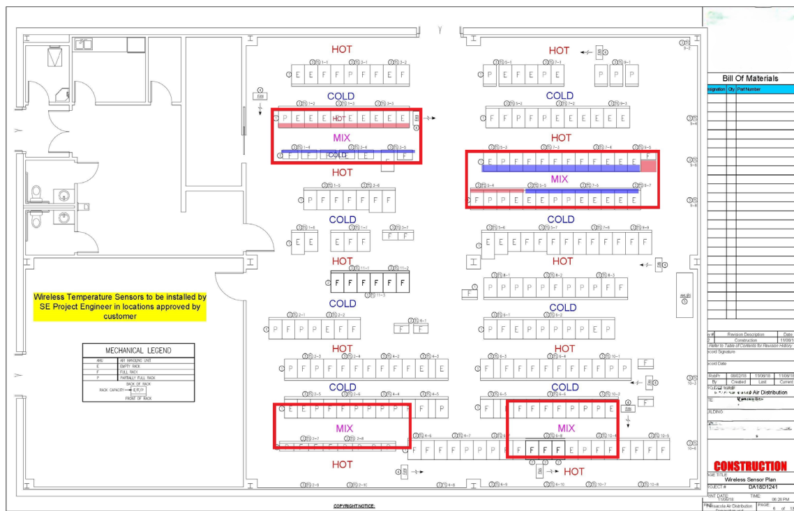
Figure 1 - “Mixed” Aisles Within Hot Aisle/Cold Aisle Setup
