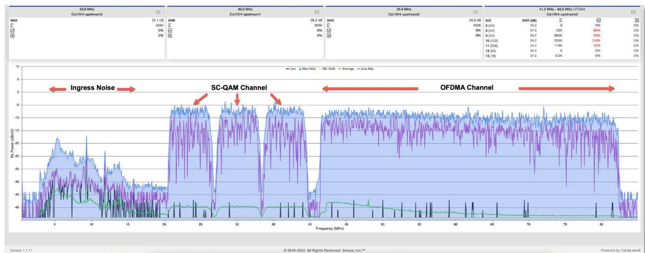
Figure 5 - Return Spectrum as Captured by UTSC
