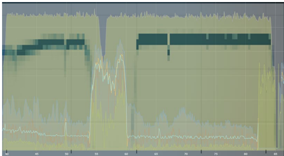
Figure 15 - An Upstream OFDMA Channel with VHF OTA Ingress and Modem RxMER Value Superimposed
