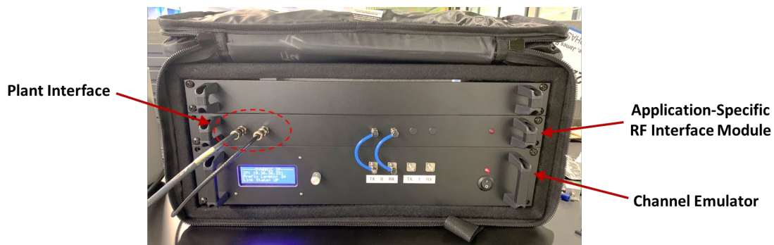
Figure 10 - Channel emulator and interface module in rack mount enclosure.
