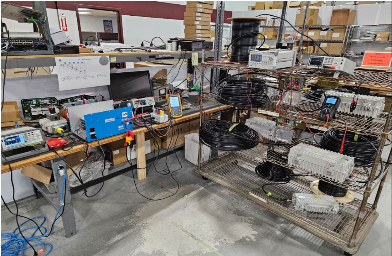
Figure 9 – 5-Amplifier Cascade Performance Testing Set-up - Picture
