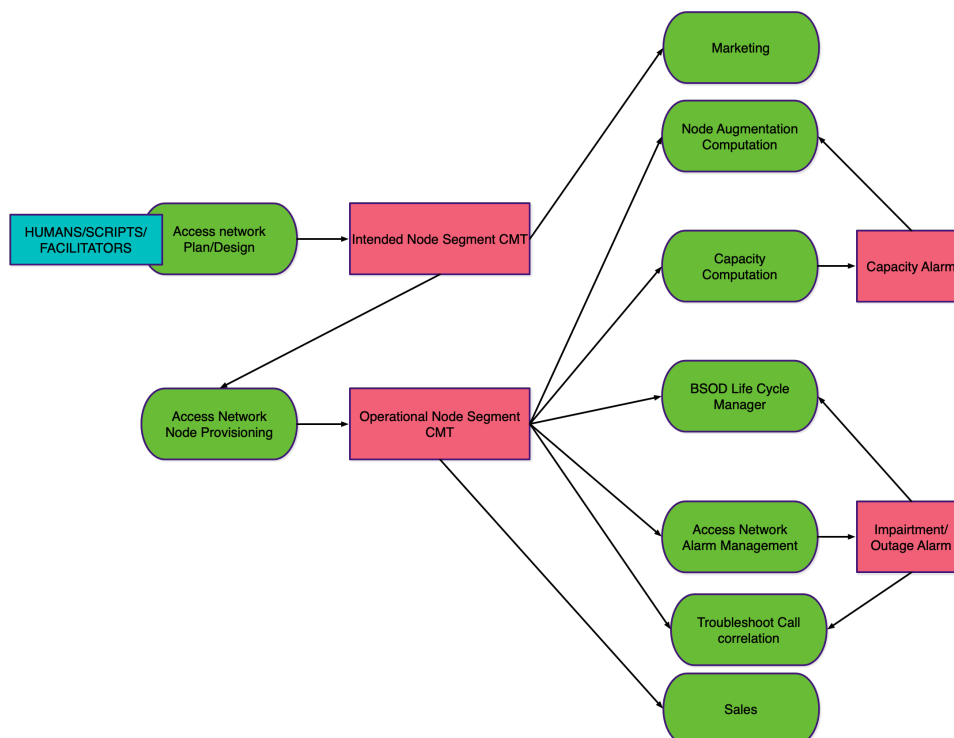
Figure 4 - Schematic illustration of how an operational digital twin can be created for many use cases and problems.
