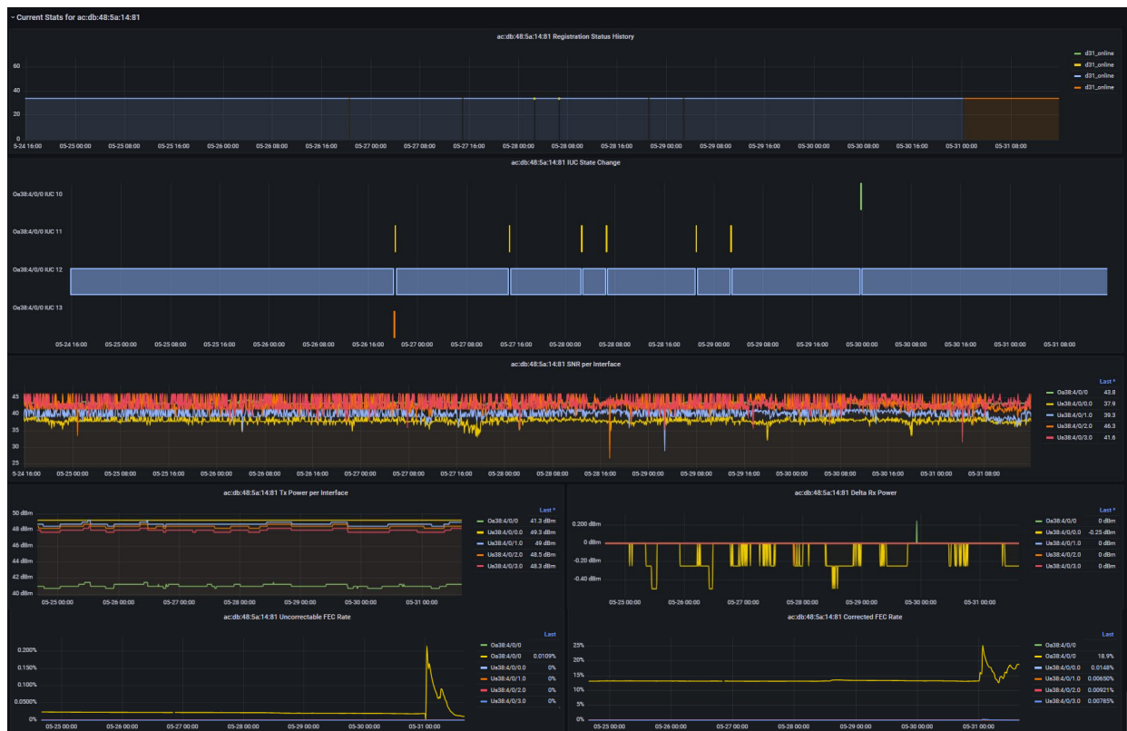
Figure 11 – Grafana Dashboard Showing CPE Characteristics
