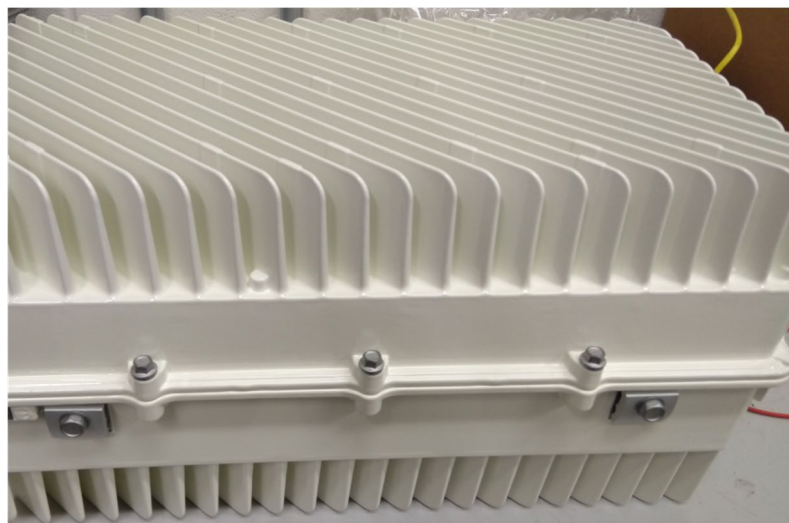
Figure 13 - Remote OLT Node Enclosure
