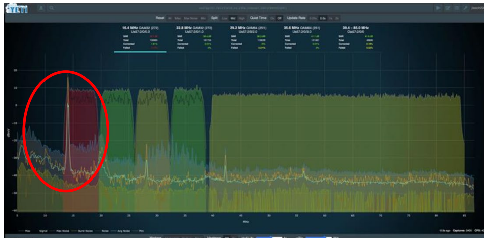
Figure 20 – High-energy narrow band interference at burst receiver, around 15 MHz
