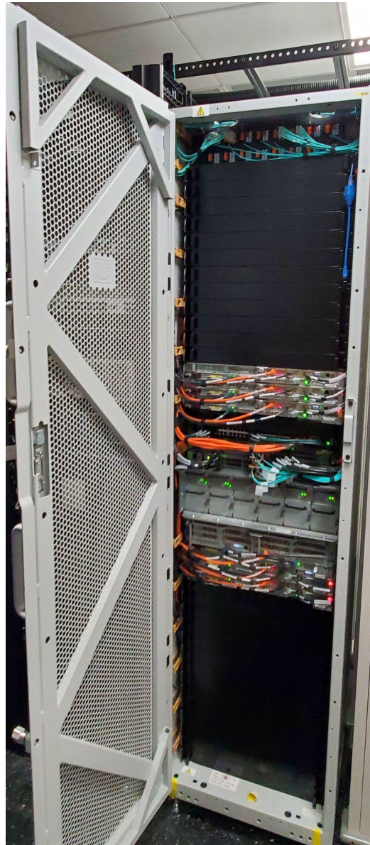
Figure 10: AWS Outpost Inside View Showing Installed RUs
