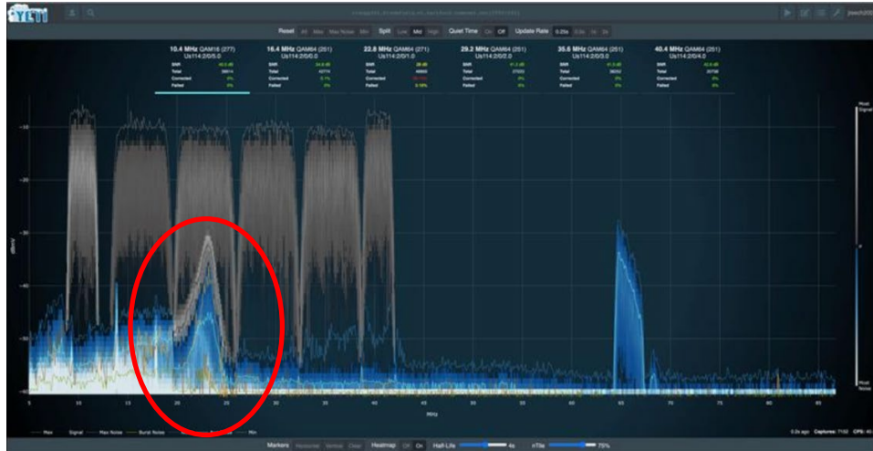
Figure 12 – Common mode disturbance at burst receiver, around 24 MHz
