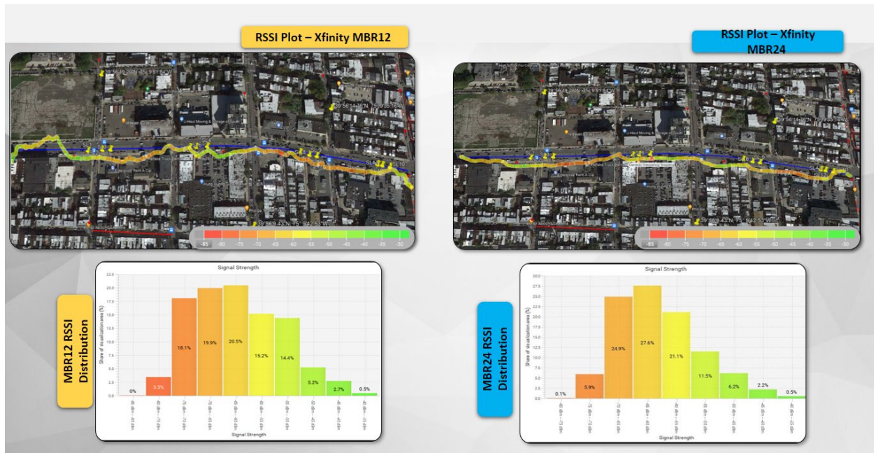
Figure 4 – Urban Ekahau Plot – Signal Strength
