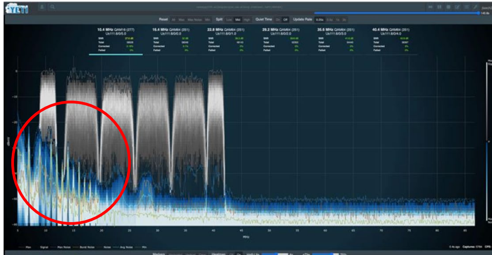
Figure 18 – Powerline gap noise at the burst receiver, below 25 MHz
