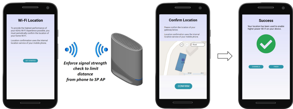
Figure 8 – Use of Smart Phone To Determine SP Device Location
