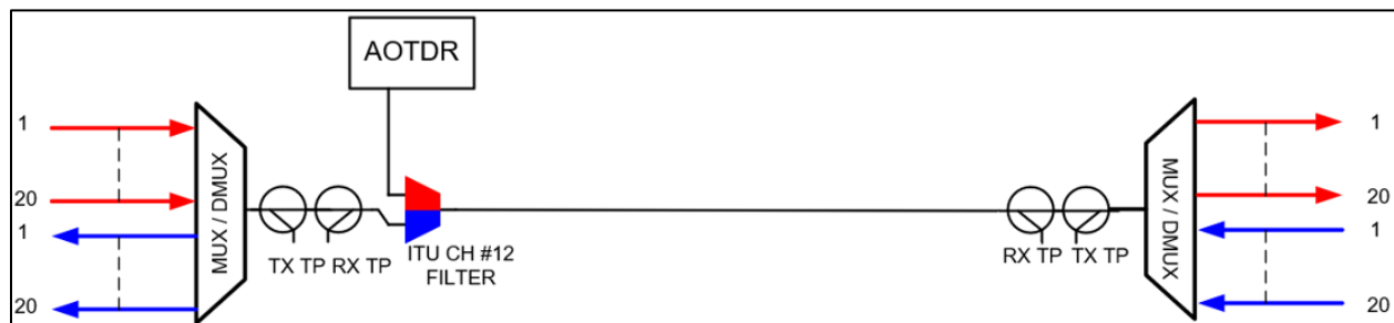
Figure 10 – Unprotected Bi-Directional Single-Fiber System
