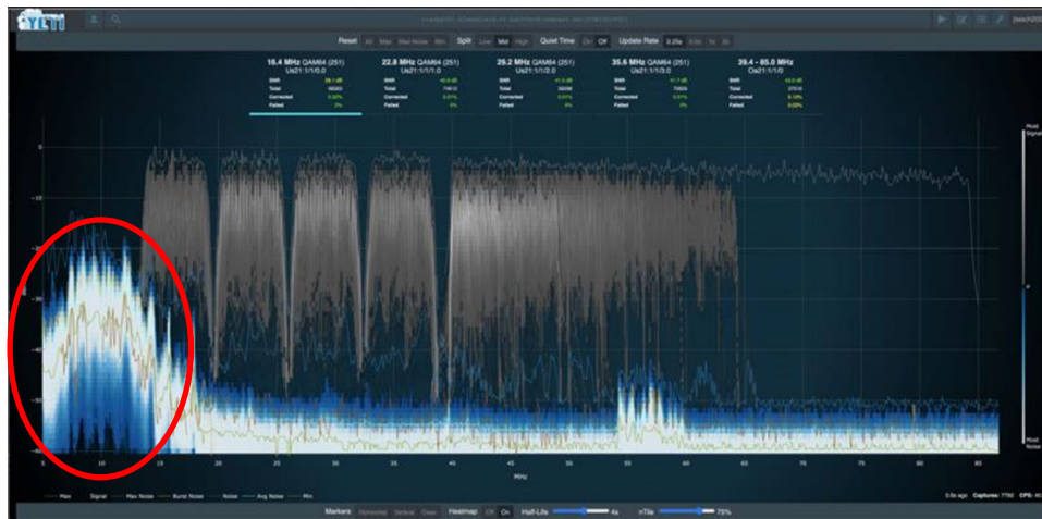
Figure 14 – Switching regulator noise at the burst receiver, centered around 10 MHz
