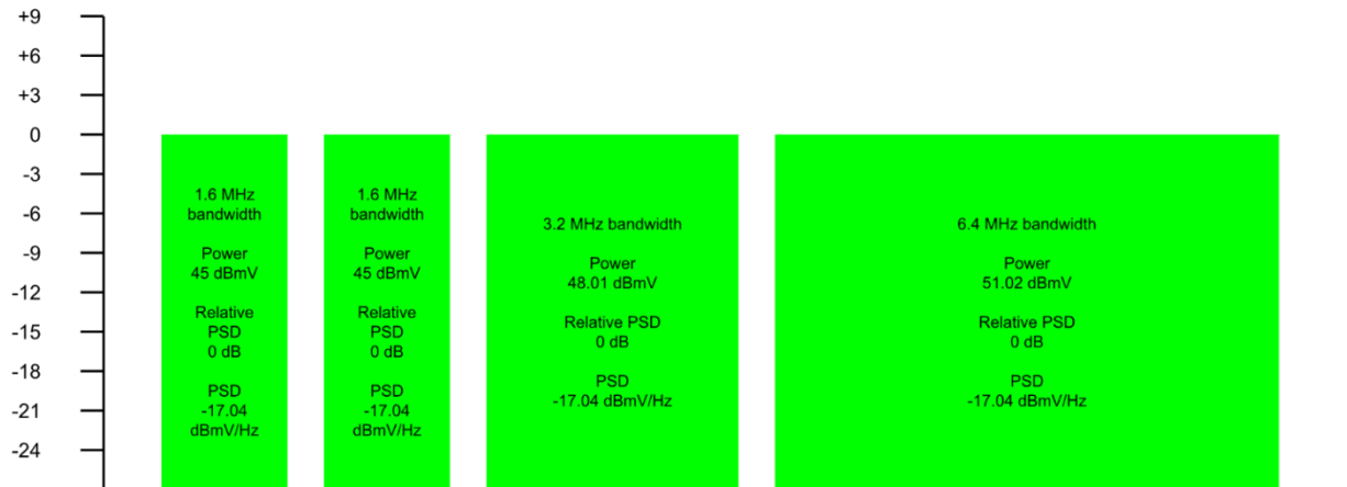
Figure 19 - Example showing four SC-QAM channels with different bandwidths but identical PSD.
