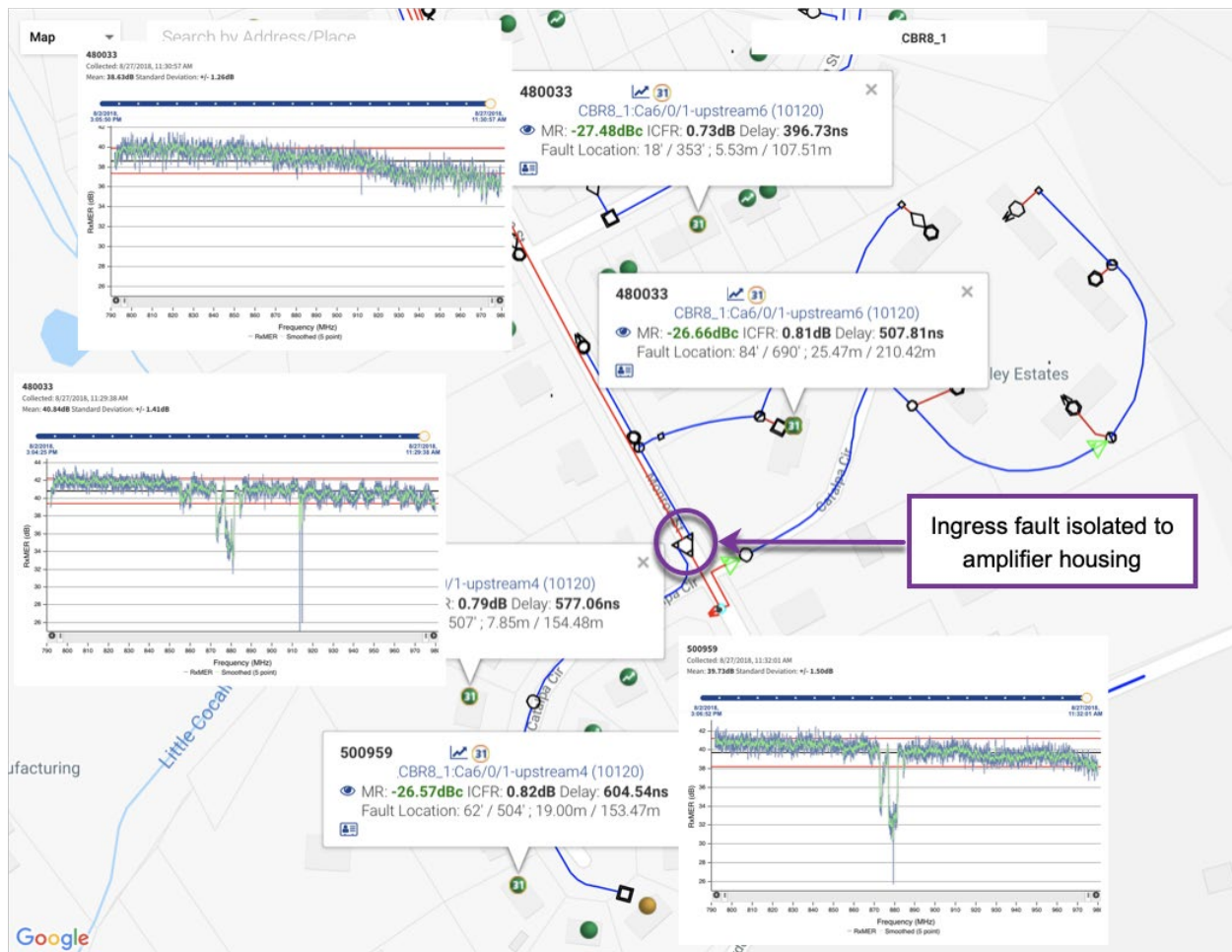
Figure 6: Localizing ingress faults using RxMER per subcarrier data (courtesy Akleza)
