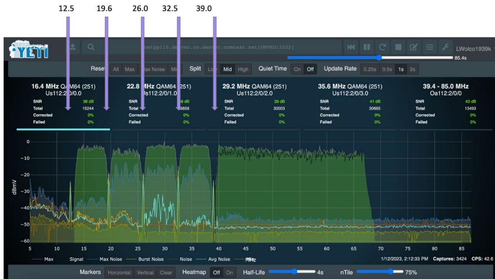
Figure 10 – Injected tones measured at the upstream burst receiver
