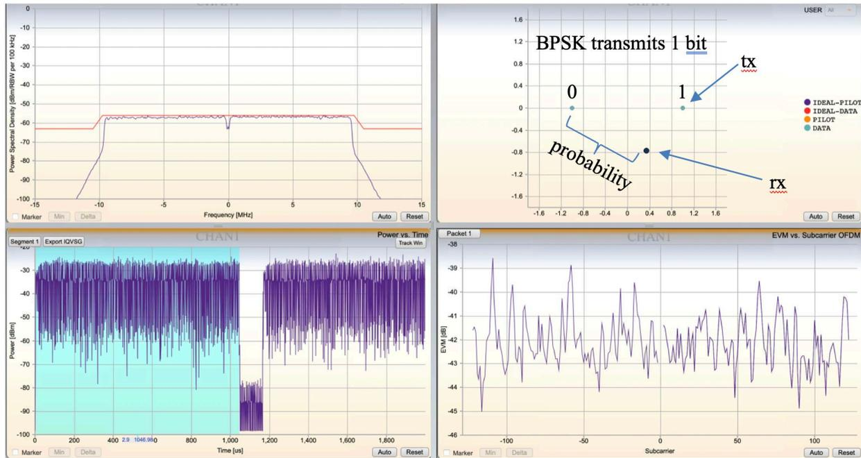
**Figure 11 – BPSK signal showing spectrum, constellation, time domain signal, EVM.**
