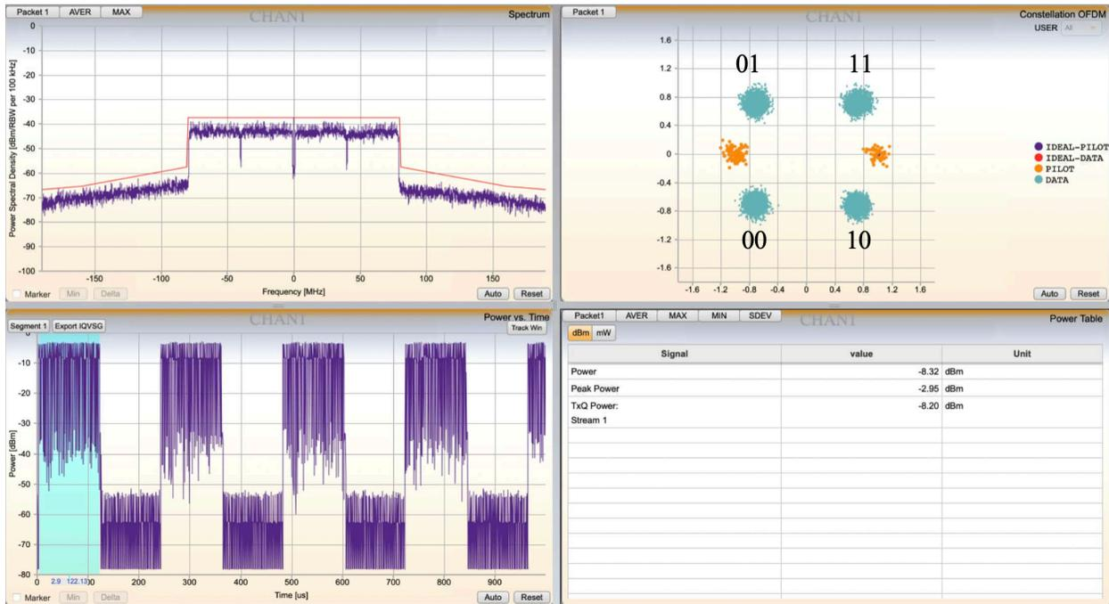
Figure 12 – QPSK modulation maps 2 bits to each subcarrier.
