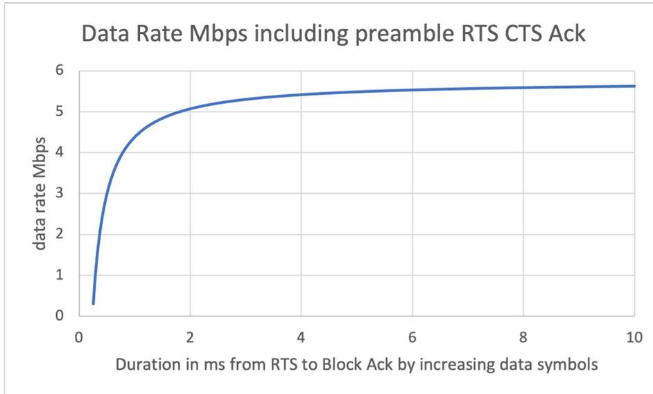
**Figure 15 – 2x2 320 MHz EHT device data rate including impact of preamble and RTS CTS Block Ack**
