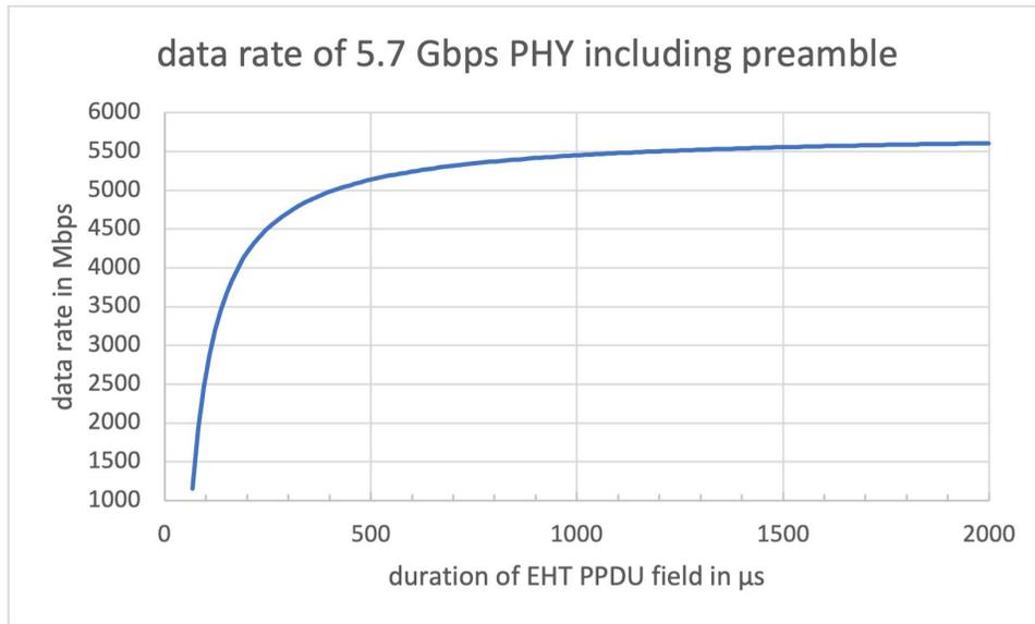
Figure 14 – 2x2 320 MHz EHT device data rate including impact of preamble
