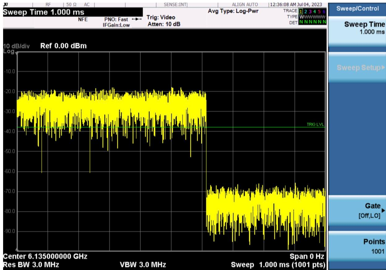
Figure 16 – The measured beacon duration of a 320 MHz 6GHz band EHT signal.
