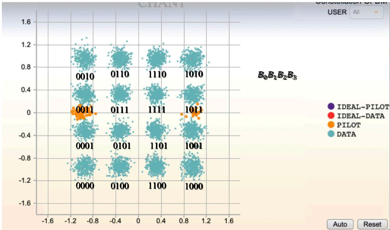
Figure 13 – 16-QAM modulation maps 4 bits to each subcarrier.
