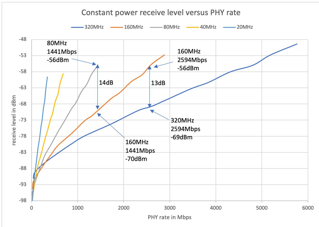
**Figure 2 – Range is improved with increased channel width for a required throughput**
