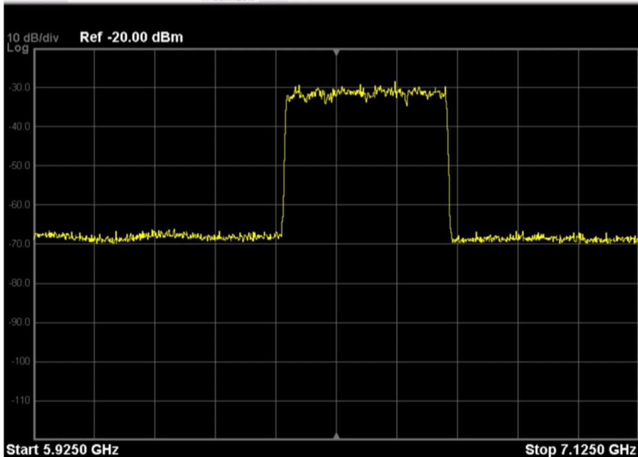
**Figure 6 – Spectrum analyzer plot of 6g133/320-2 over 6 GHz band**
