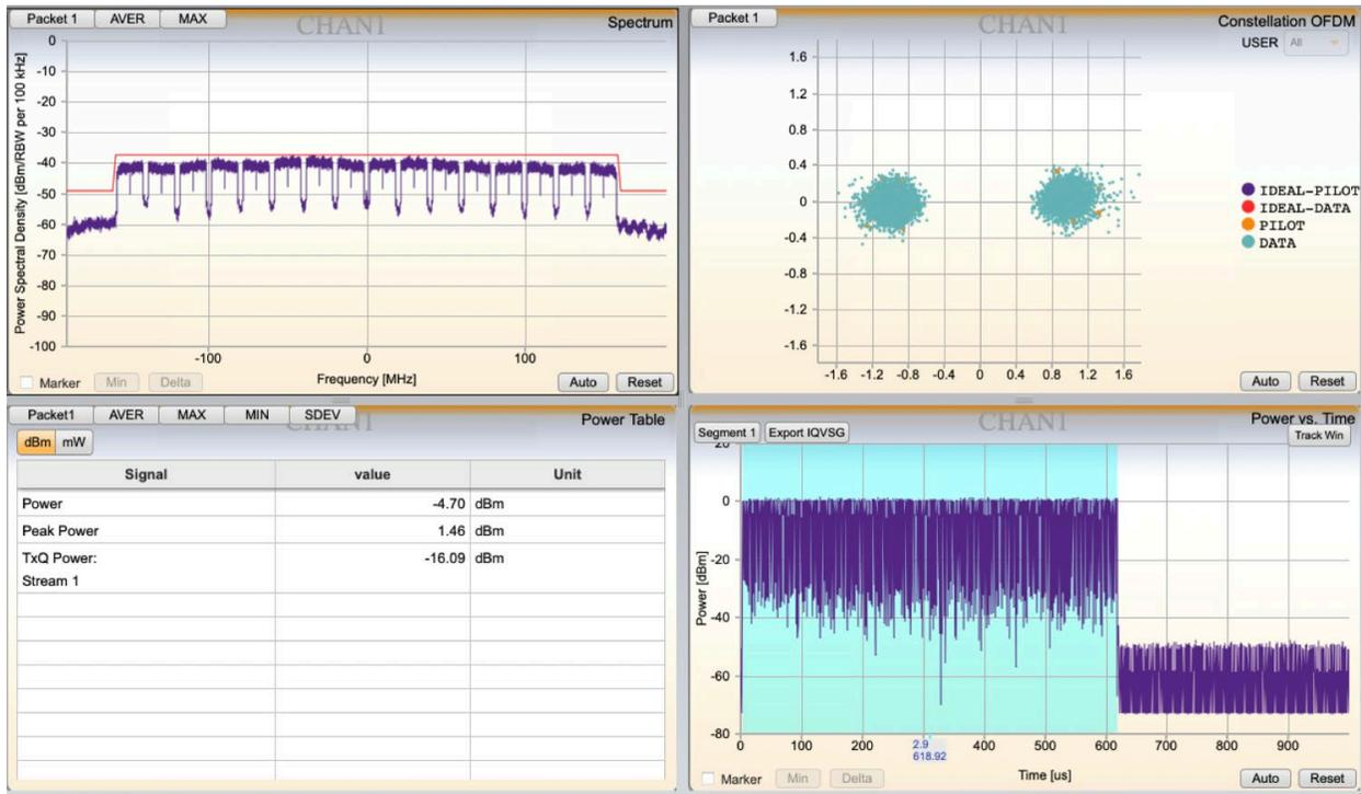
Figure 17 – The beacon is repeated over the full 320 MHz channel width
