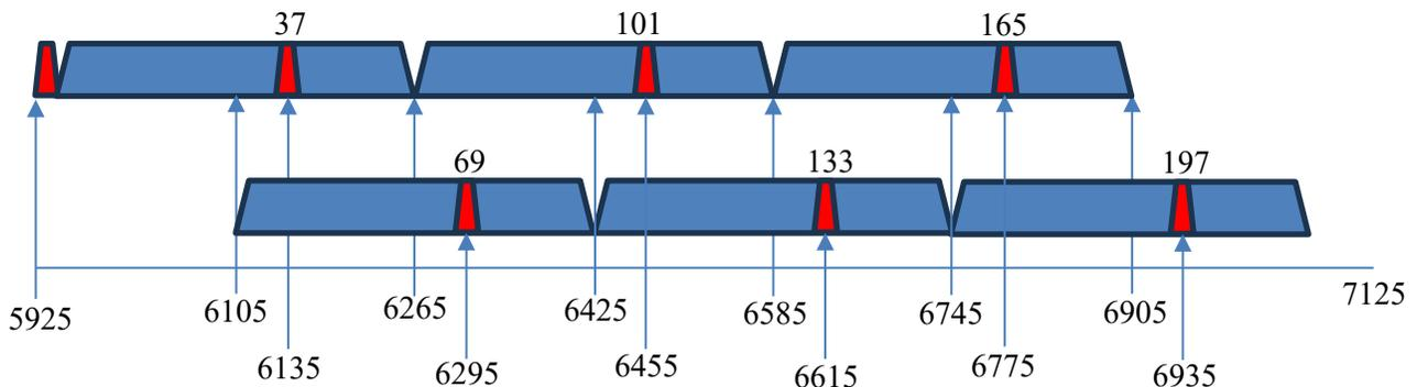
Figure 5 – 6 GHz band preferred scanning channels and center frequencies in MHz
