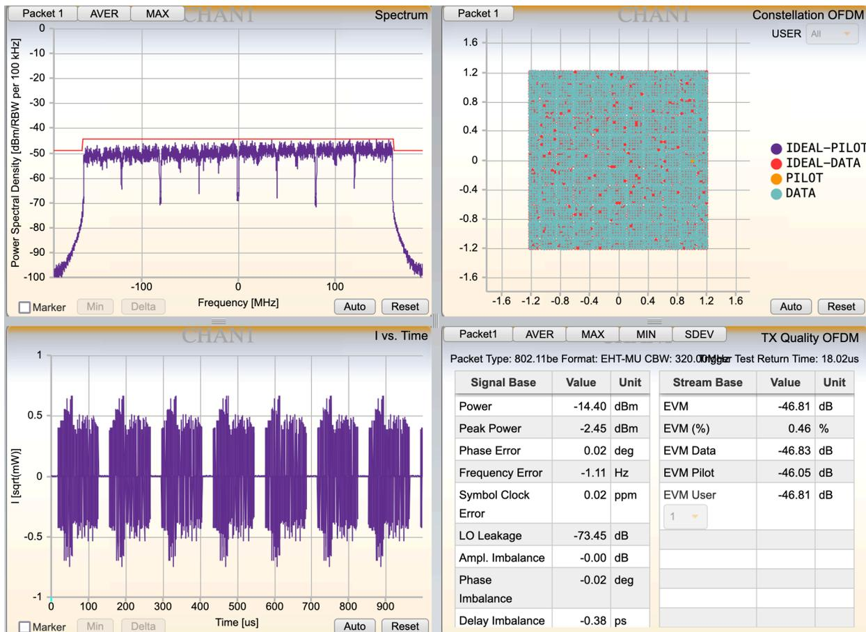
Figure 10 – MCS13 QAM-4096 LDPC 5/6 320 MHz 802.11be Wi-Fi 7 signal
