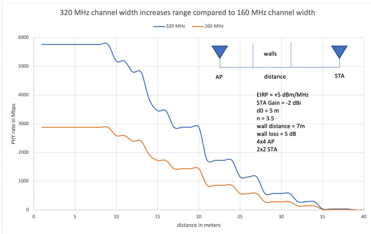
Figure 3 – Improvement in range for 320 MHz with constant power spectral density
