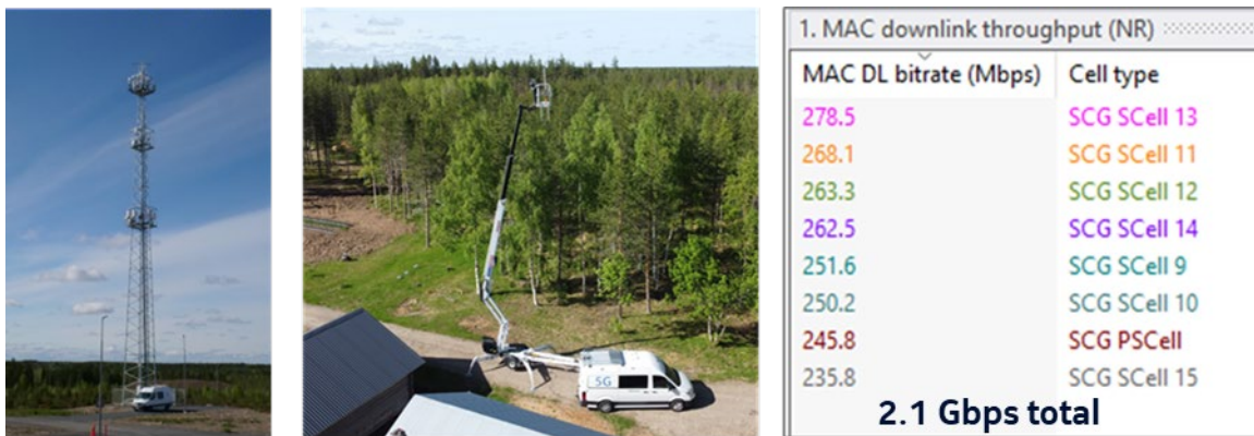
Figure 18 – Field trial results for 11 km extended range mmWave site
