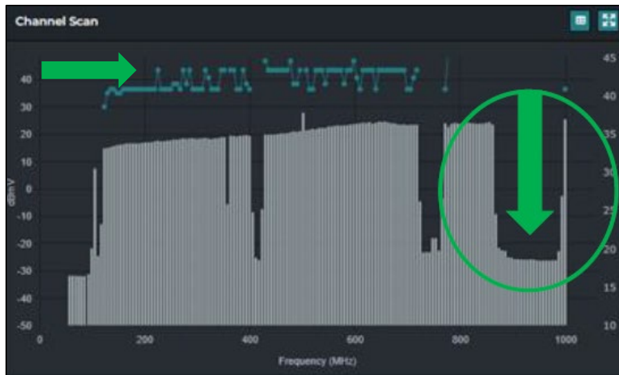
Figure 8- Same Amplifier When Properly Aligned
