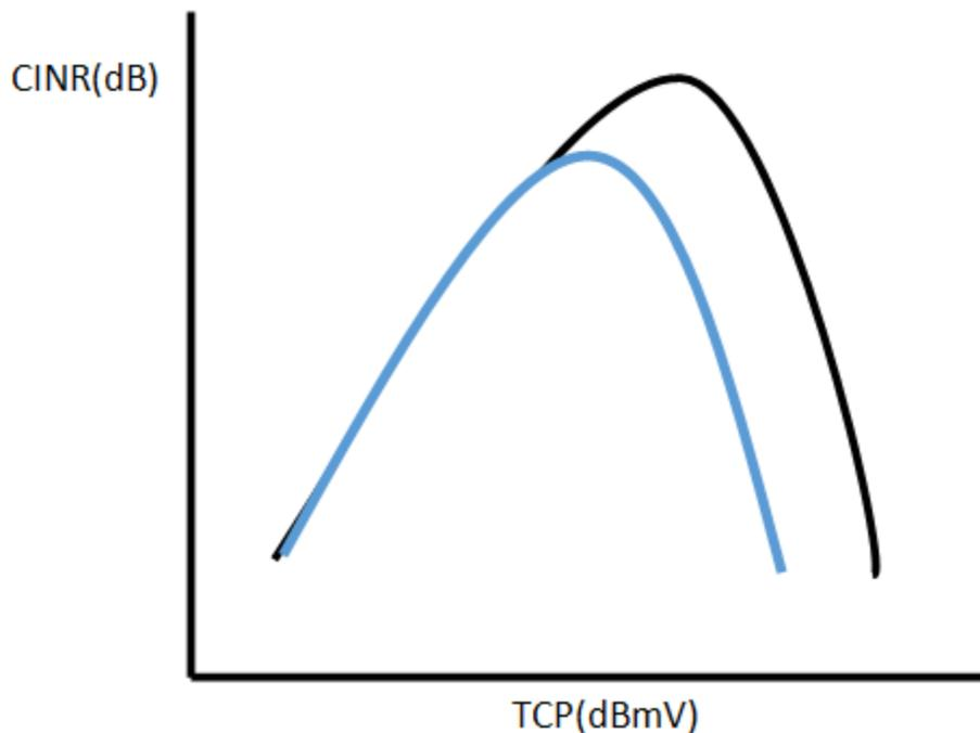
**Figure 17 – Example Amplifier CINR Curve**
