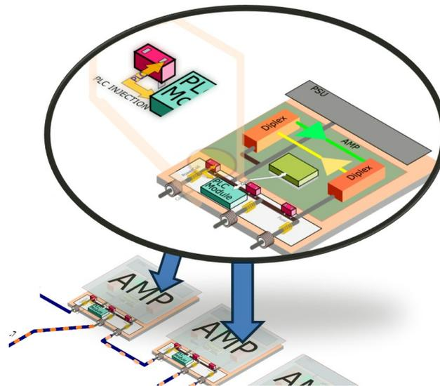
**Figure 7 – PLC Implementation in HFC Amplifiers**
