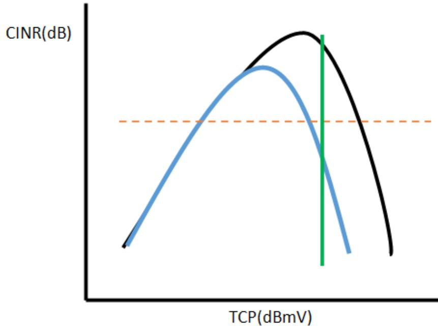
Figure 18 – Amplifier CINR and Required TCP – Full Channel Loading
