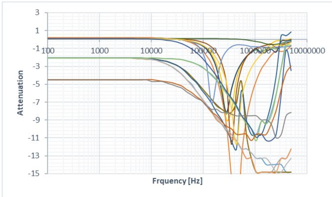
Figure 9 – Insertion Loss of 20 Different Passive Devices from 100 Hz to 5 MHz
