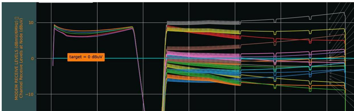
Figure 16 – The Same System Operating at 492 MHz Split – Post Optimization
