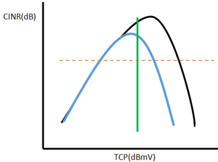
Figure 19 – Amplifier CINR and Required TCP – Reduced Channel Loading
