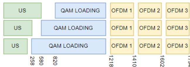
Figure 14 – Channel Loading Examples for Various Splits
