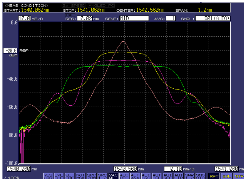
Figure 8 – Modulated linewidth at different data rates and modulation orders
