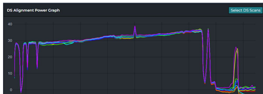
Figure 1 - A clean, linear frequency full band capture response
