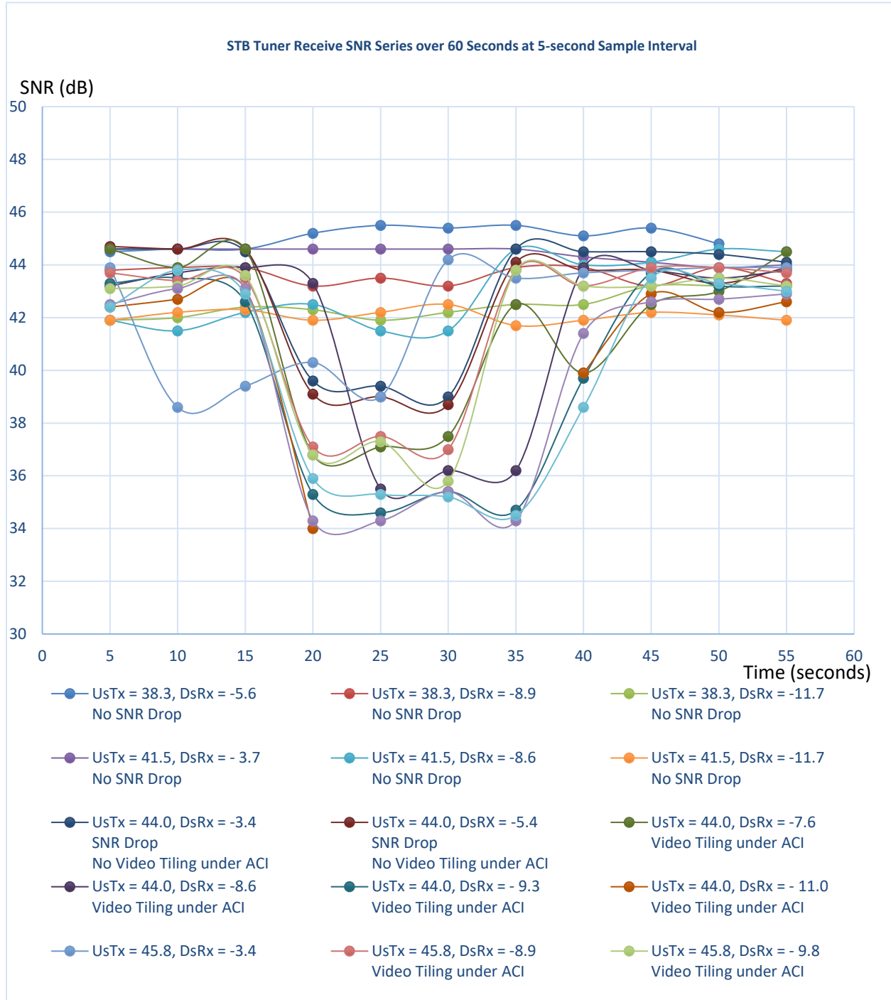
Figure 14: Model-C Tuner SNR Sample Series Under Different Rx and HS-CM Tx Power Levels
