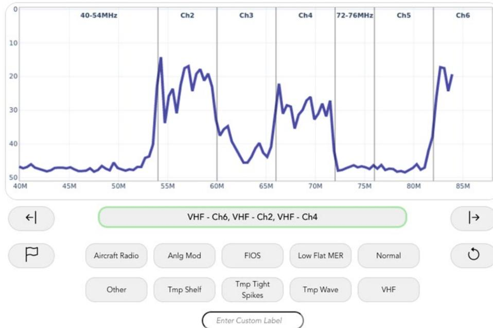
**Figure 8 - Example of an MER plot in the labeling tool. The tool is used to both assign initial labels and conduct periodic reviews of the model’s predictions.**
