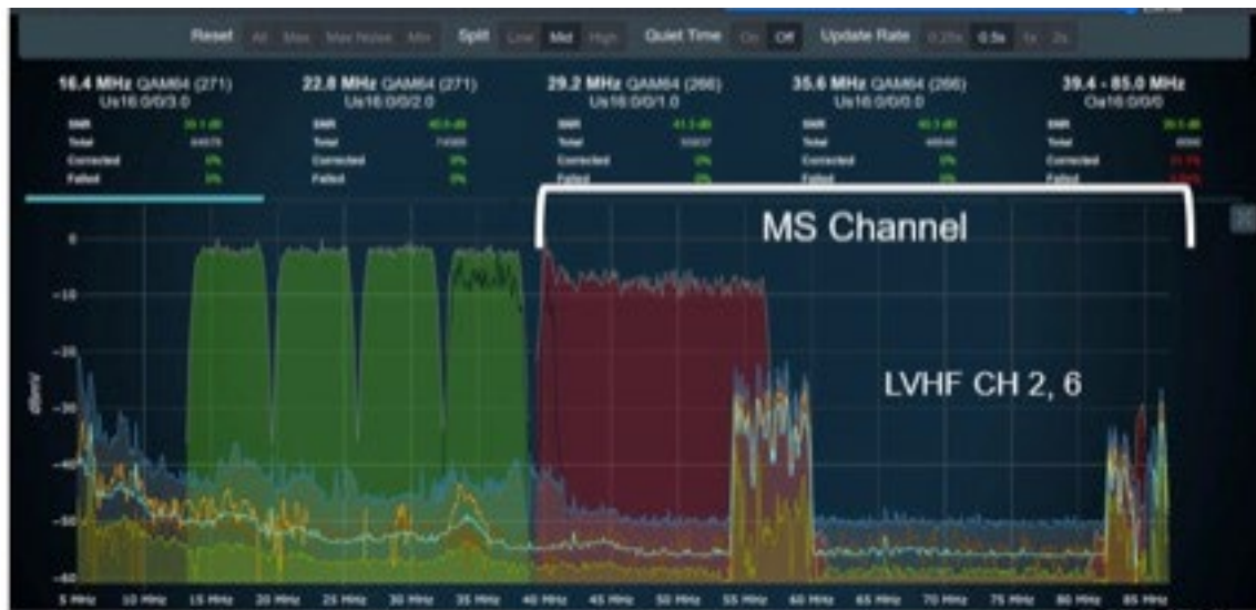
Figure 9: Lower VHF ingress into mid-split channel would have required 32-QAM or lower modulation without PMA solution.
