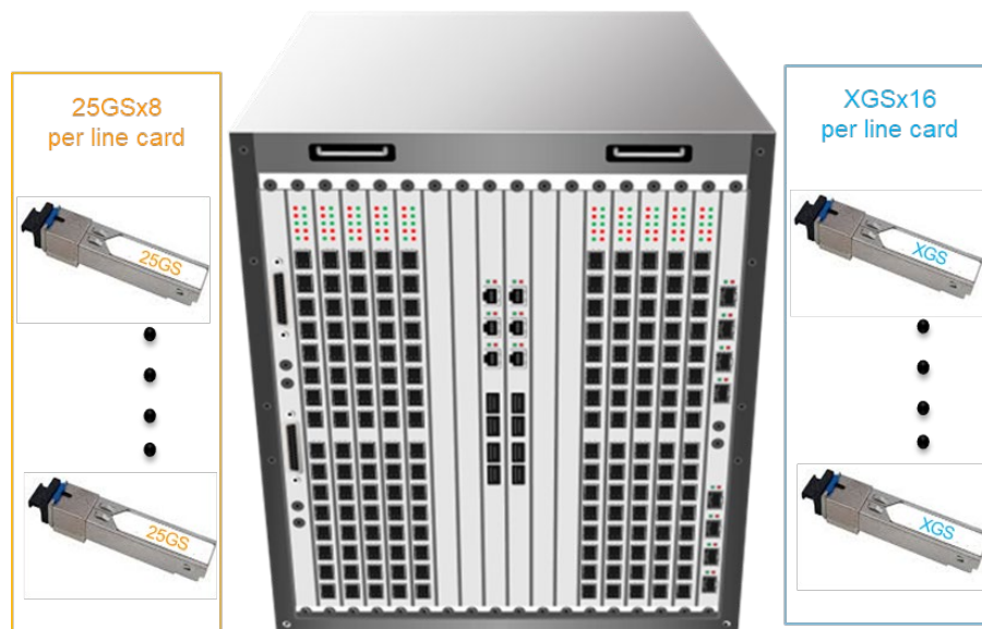
Figure 7 – Example of Chassis with Dual Speed XGS/25GS Line Cards
