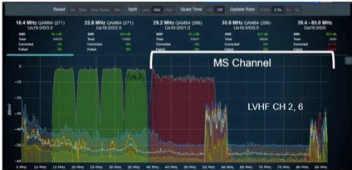
Figure 9: Lower VHF ingress into mid-split channel would have required 32-QAM or lower modulation without PMA solution.
