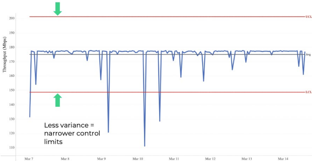
Figure 12 - Control Chart of CM DS Speed Test of Higher Stability Service
