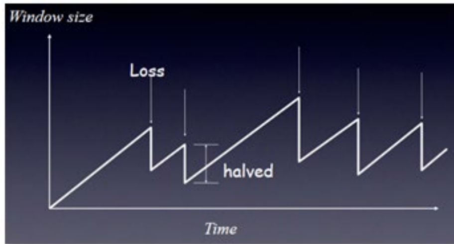
Figure 4 - Bandwidth Usage for Capacity Seeking Applications with TCP
