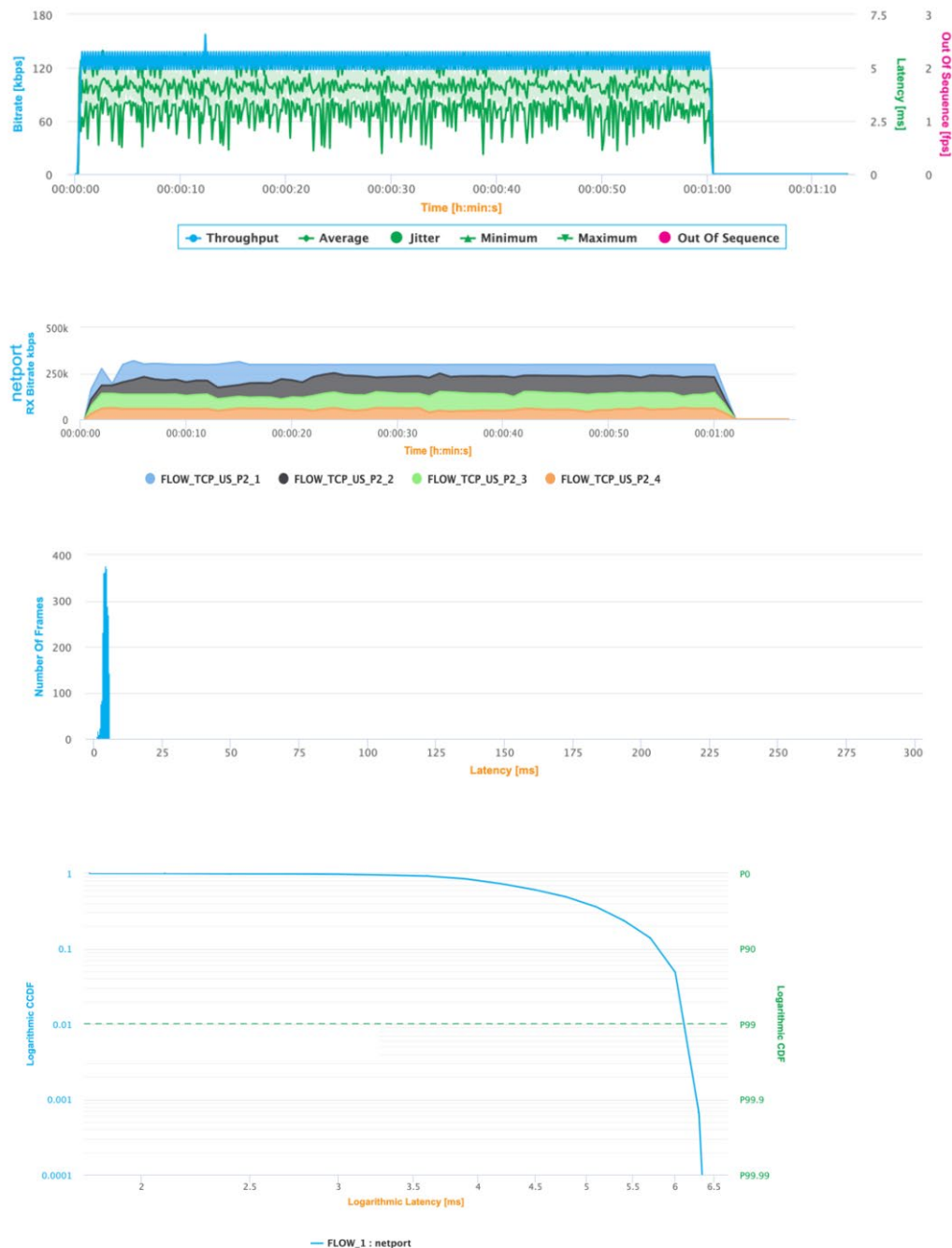
Figure 8 – Latency statistics for US LLD example with PGS
