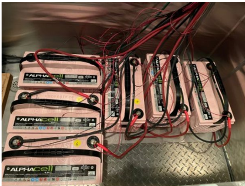
Figure 5 – Tested Batteries for Temperature Effect
