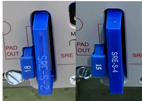
Figure 12 – Sub-split return equalizers installed in mid-split amplifiers
