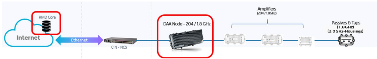
Figure 22 – Step 4: DOCSIS 4.0 High Split
