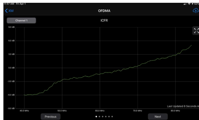
Figure 13 – Frequency response of OFDMA channel through a sub-split equalizer
