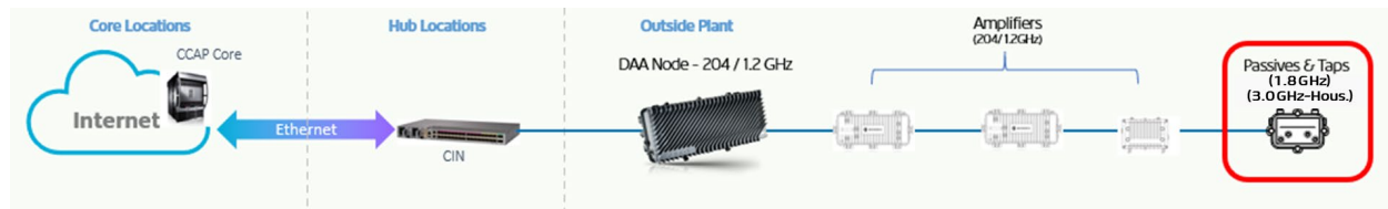
Figure 20 – Step 2: D3.1 High Split with 1.8 GHz Taps (in 3.0 GHz Housings)
