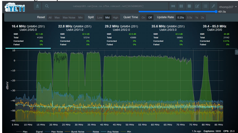
Figure 5 – Probe Signal Used in iHAT via DOCSIS 3.1 OUDP Feature
