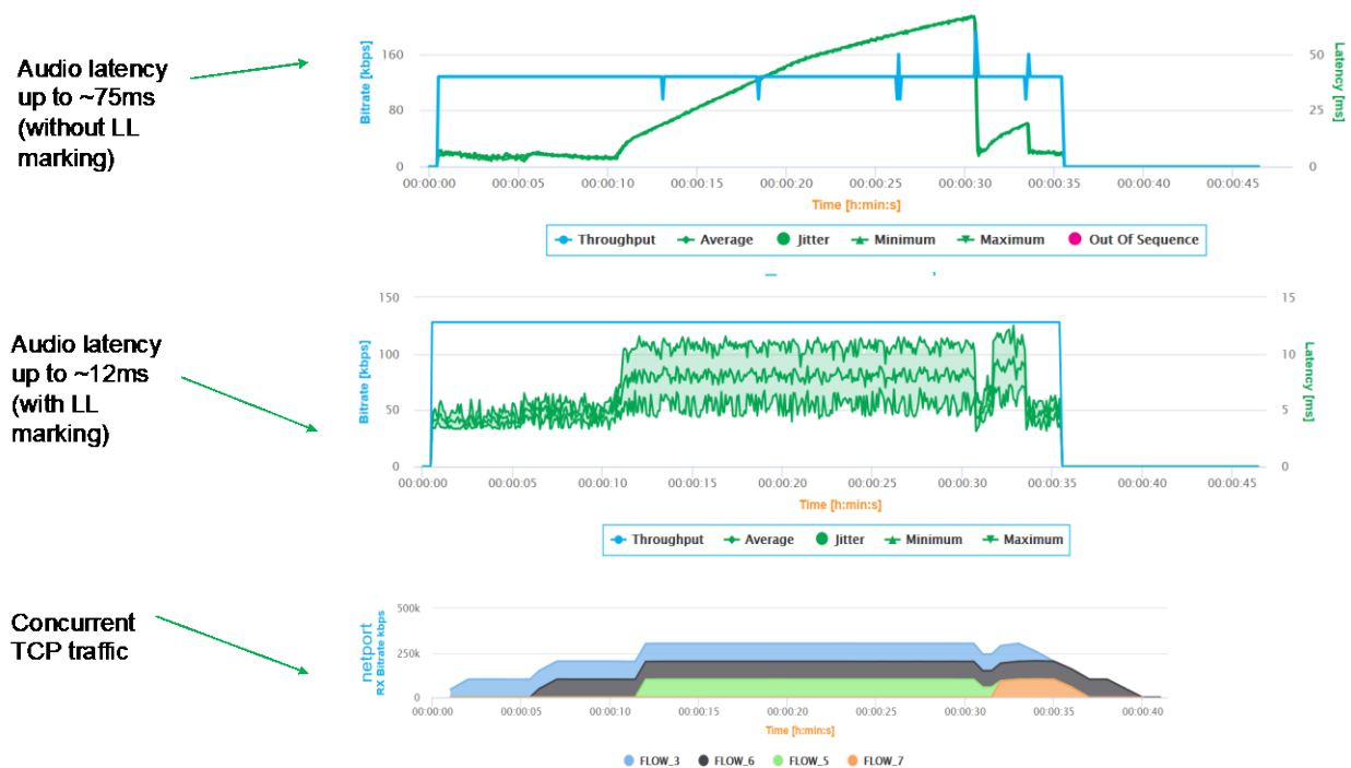
Figure 3 – US LLD example showing the impact of QB traffic on NQB traffic latency
