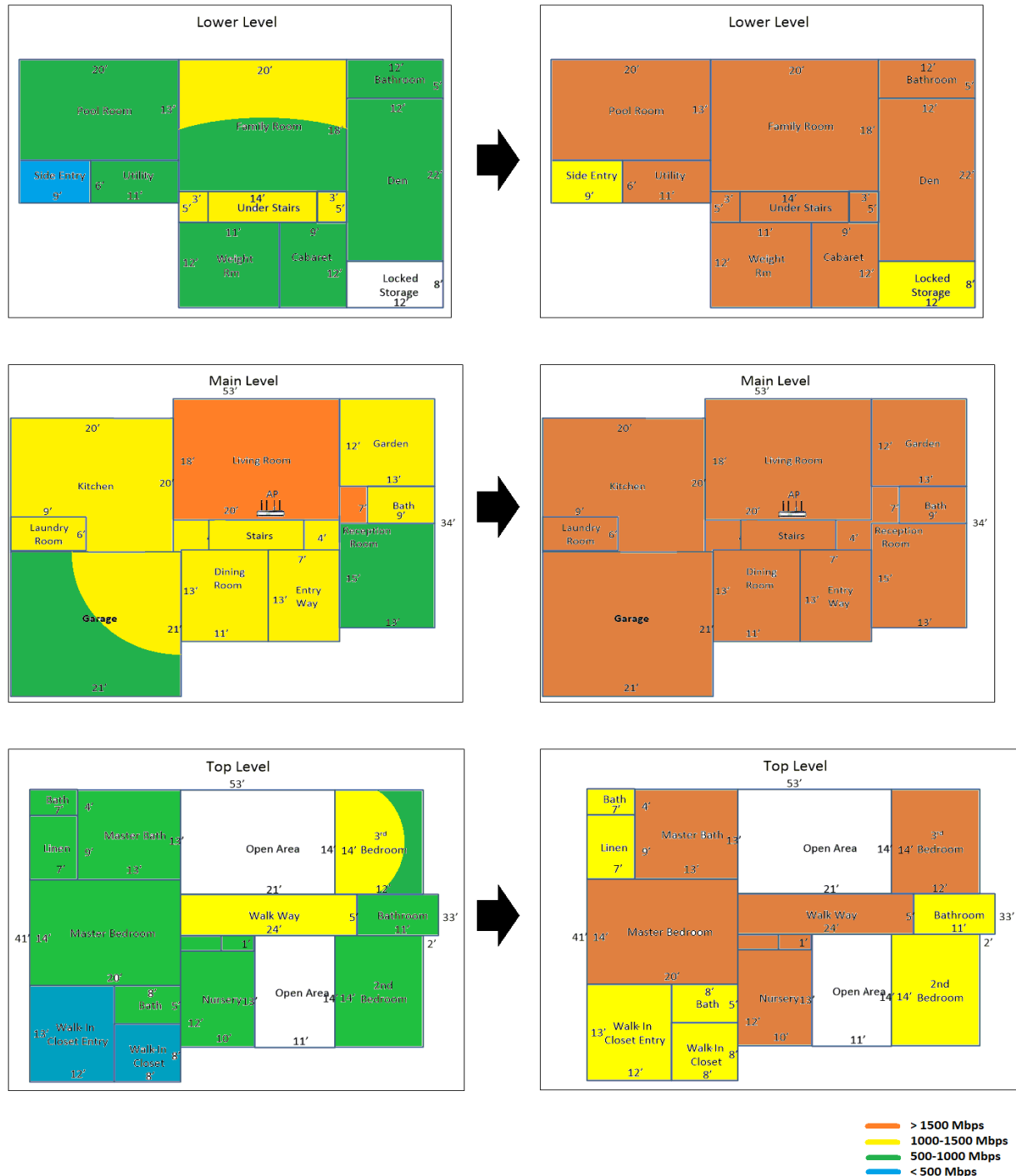
Figure 1 – Standard Power Benefit over LPI at 6 GHz in Arris Wi-Fi House
