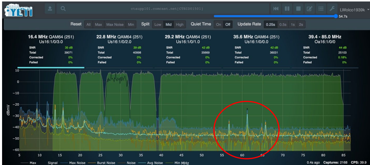
Figure 21. Example video modulator in home transmitting into OFDMA spectrum
