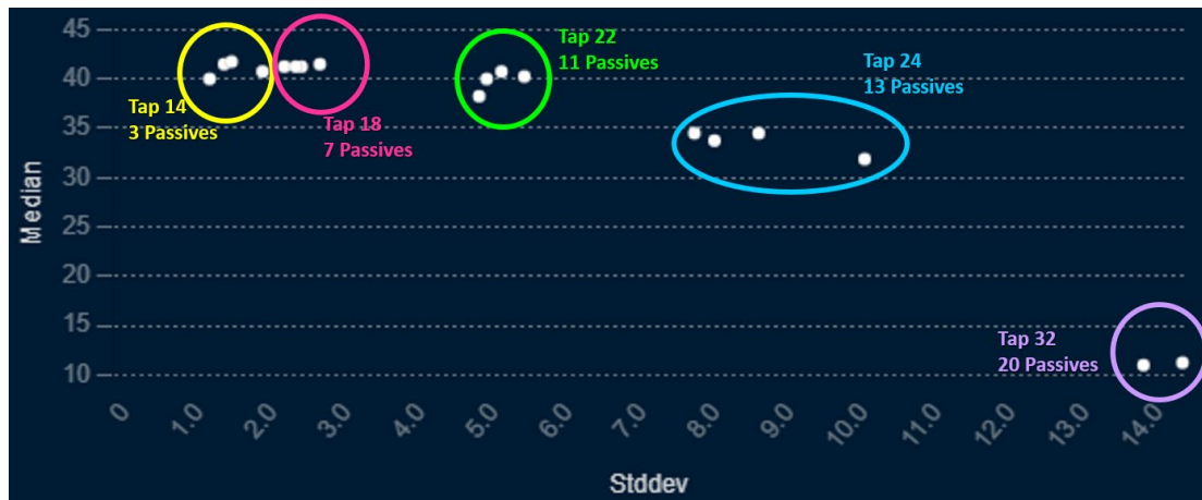
Figure 23. Median vs Standard Deviation for CM across the HFC plant
