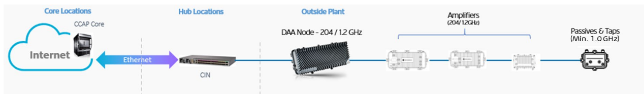
Figure 19 – Step 1: D3.1 High Split (204 MHz / 1 GHz)
