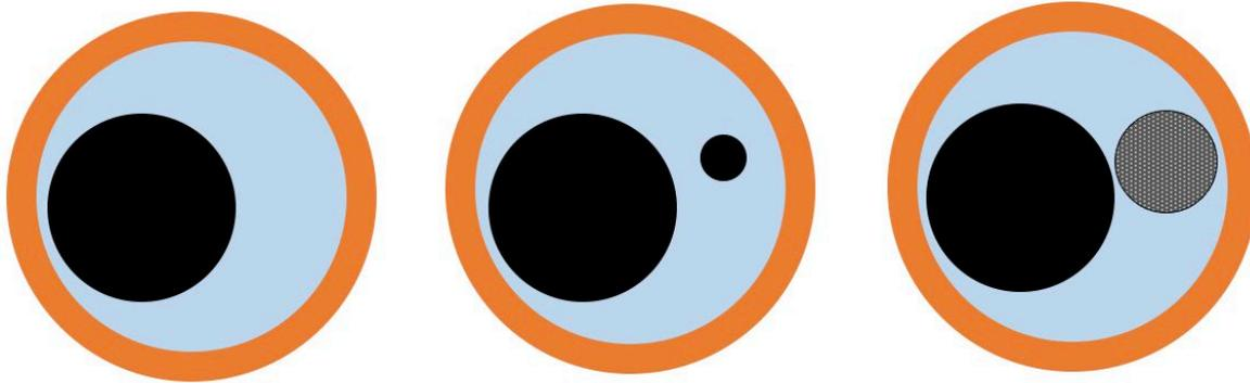
**Figure 5 – Illustrating CiC Linear and Area Fill Ratios for various cables**
