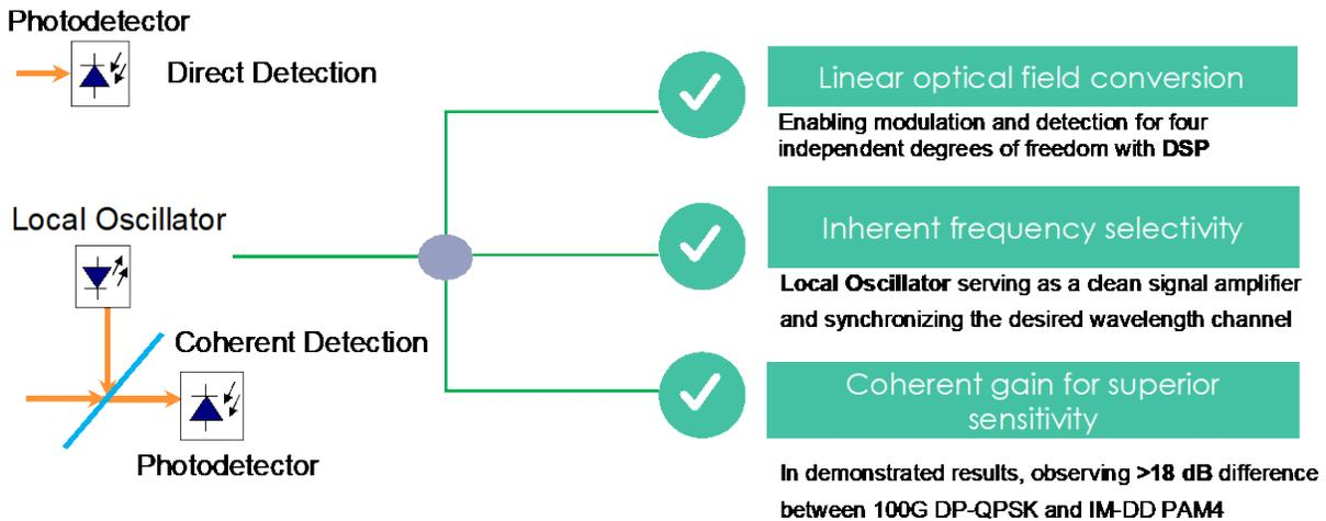
**Figure 3 – Technology Comparison: Coherent Optics vs. IM-DD**
