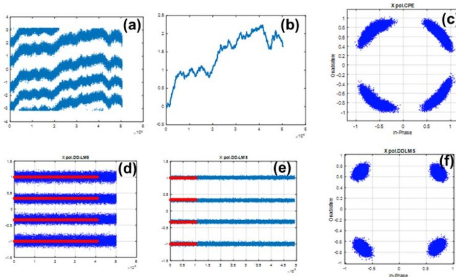
**Figure 7 – Signal in Different Stages of Receiver-side DSP Process. (a) optical signal phase after frequency-offset estimation; (b) estimated optical signal phase noise; (c) QPSK signal constellation without phase domain equalization; (d) corresponding phase of QPSK signal in (c) mapped back to PAM-4 signals; (e) equalized PAM-4 signals after phase domain post-equalization; (f) QPSK signal constellation with phase domain equalization.**
