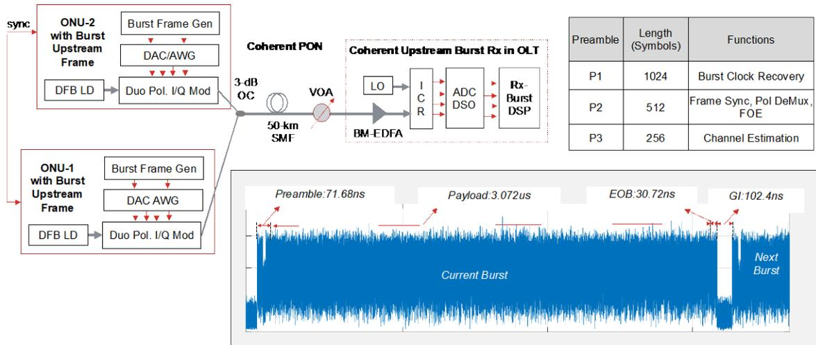
**Figure 13 – Experimental Verifications for Coherent Burst System**
