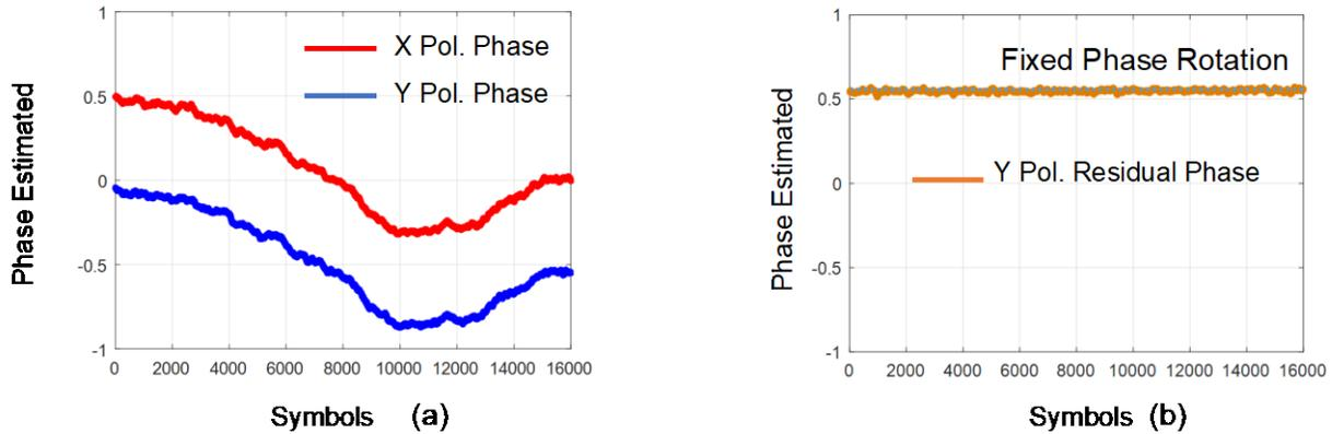
**Figure 10 – Phase Estimation Results for Two Polarizations**
