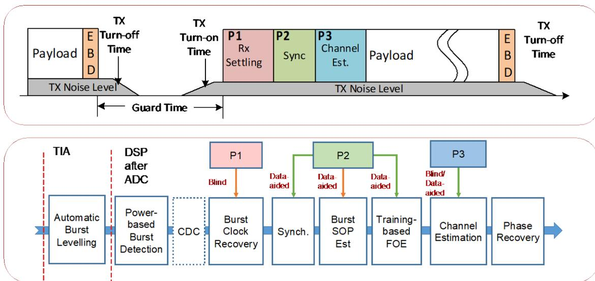
**Figure 12 – Preamble Design and Coherent Burst Signal Processing**
