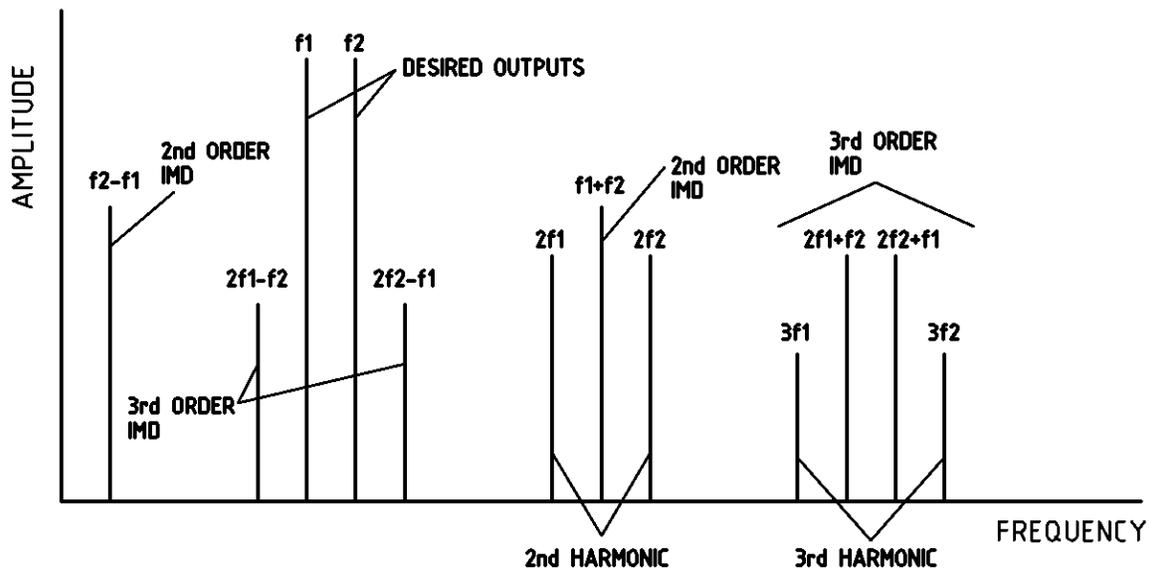
**Figure 2 – 2<sup>nd</sup> and 3<sup>rd</sup> order spectral components created by sine waves at  $f_1$  and  $f_2$ .**
