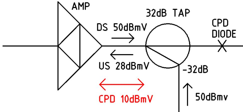
**Figure 6 – CPD non linear distortions in downstream**
