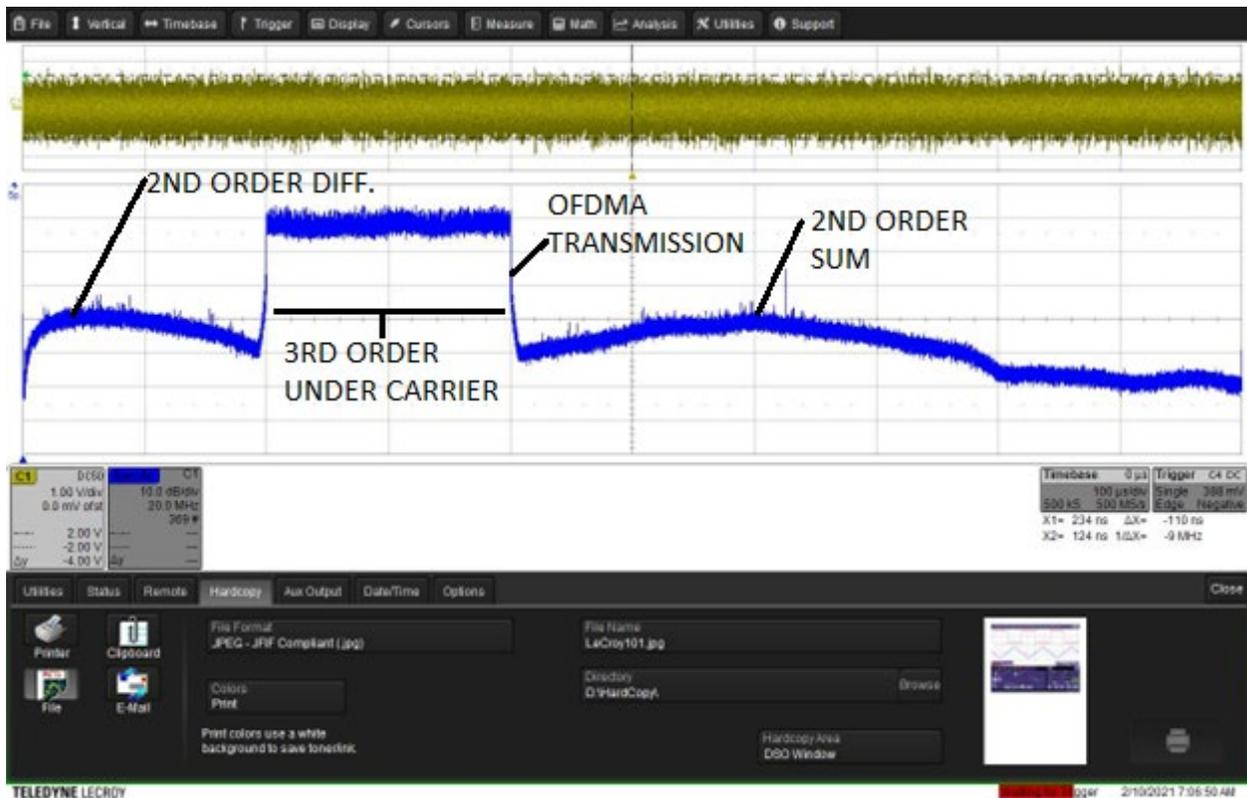
**Figure 9 – OFDMA spectral plot (Shunting corrosion diode)**
