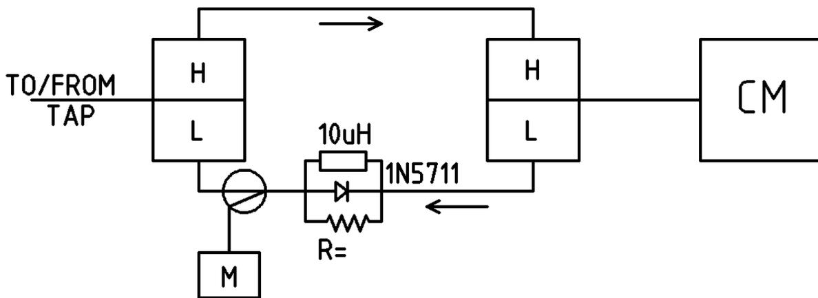
**Figure 7 – Circuit simulation of corrosion in a drop.**
