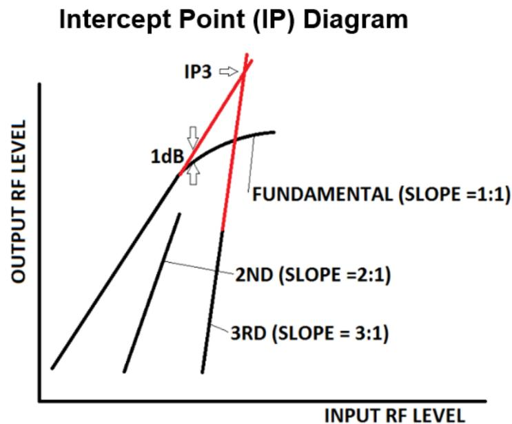
**Figure 3 – Plots of fundamental, 2<sup>nd</sup> and 3<sup>rd</sup> order distortions vs fundamental RF levels.**
