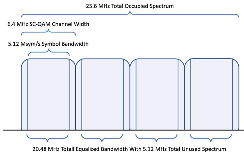
**Figure 1 – Example of SC-QAM equalized spectrum**
