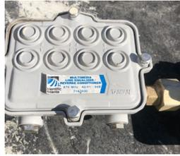
**Figure 10 – Conditioned line equalizer**
