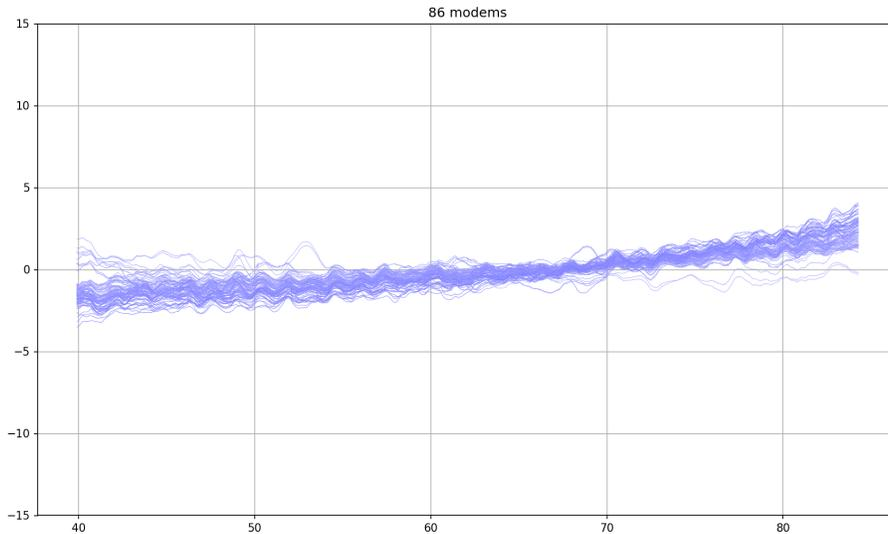
**Figure 4 – Multiple modems' pre-equalizer amplitudes on a node**
