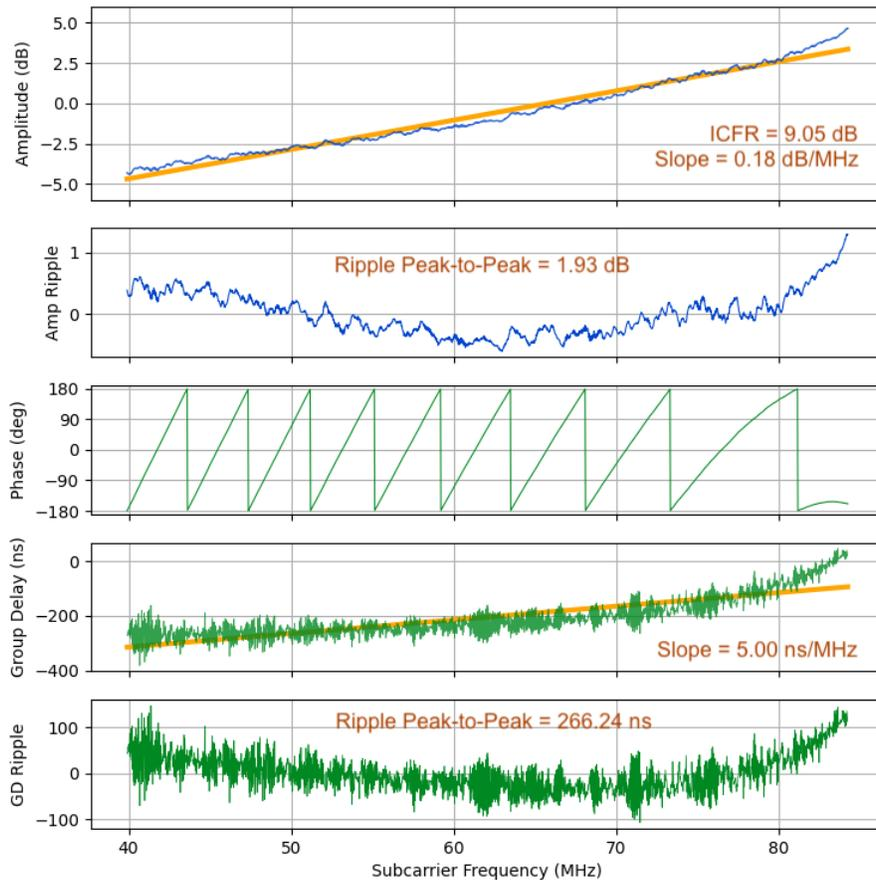
**Figure 3 – Example of OFDMA pre-equalizer coefficients and metrics**
