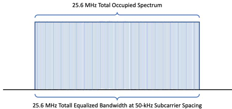
**Figure 2 – Example of OFDMA equalized spectrum**
