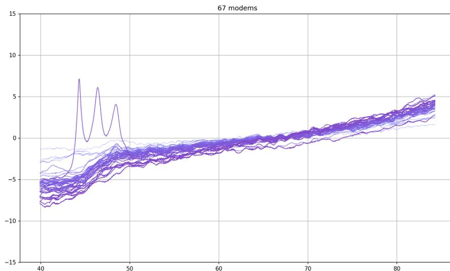
**Figure 8 – Same 12 modems' frequency reponse after repair**
