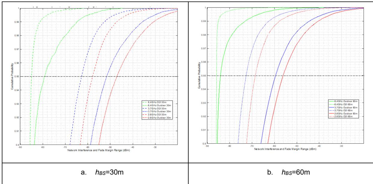
**Figure 6. Comparative network interference impact for outdoor and O2I scenarios (network load 50%, 95% service availability, Vtilt=-15°, 2.6, 3.7 and 6.4GHz),  $h_{BS}$ =30m and 60m.**
