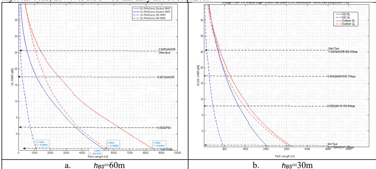
**Figure 8. Comparative DL and UL SNR for Outdoor and O2I Scenarios (3.7GHz),  $h_{BS}=60m$  vs.  $h_{BS}=30m$**
