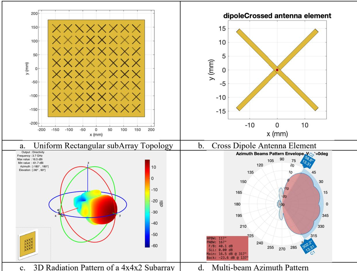
**Figure 15. Sample of BS array parameters (3.7GHz). (a) Array geometry [2 2] subarrays, (b) Cross-Dipole antenna element geometry, (c) 3D radiation of a subarray (4x4x2) and (d) multi-beam azimuth radiation pattern.**
