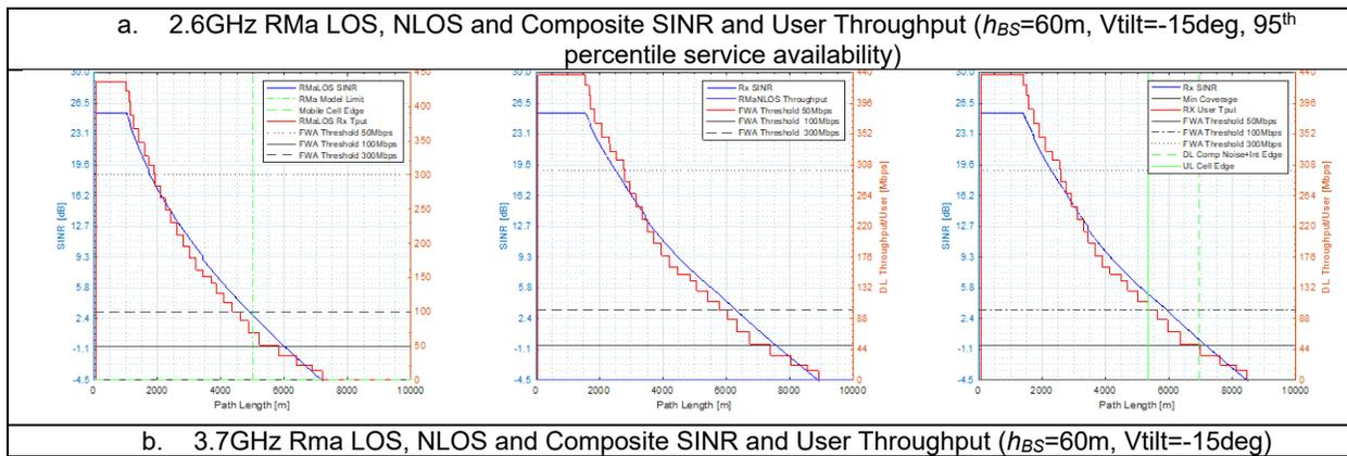
**Figure 11. Comparative LOS, NLOS and Composite SINR and Tput, 2.6 3.7GHz<sup>2</sup>**
