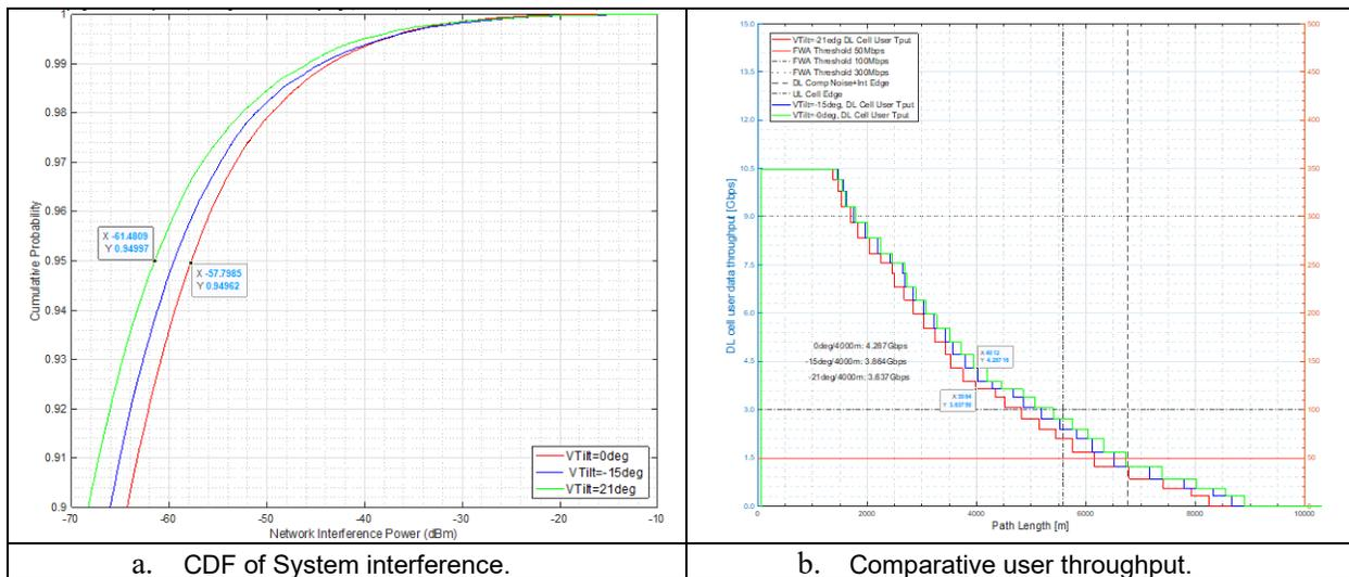
**Figure 4 Vtilt impact upon system interference and the related user throughput degradation as a function of Elevation Vtilt=0°/-15°/-21° ( $h_{BS}=60m$ , outdoor scenario, NetLoad=50%, 95% Service Availability, 3.7GHz).**
