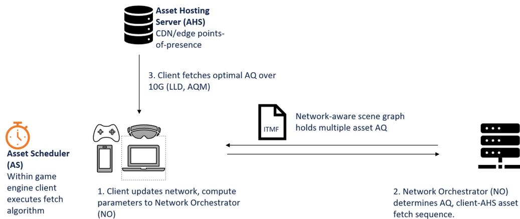
**Figure 2 - Intelligent Buffering over the 10G Network**
