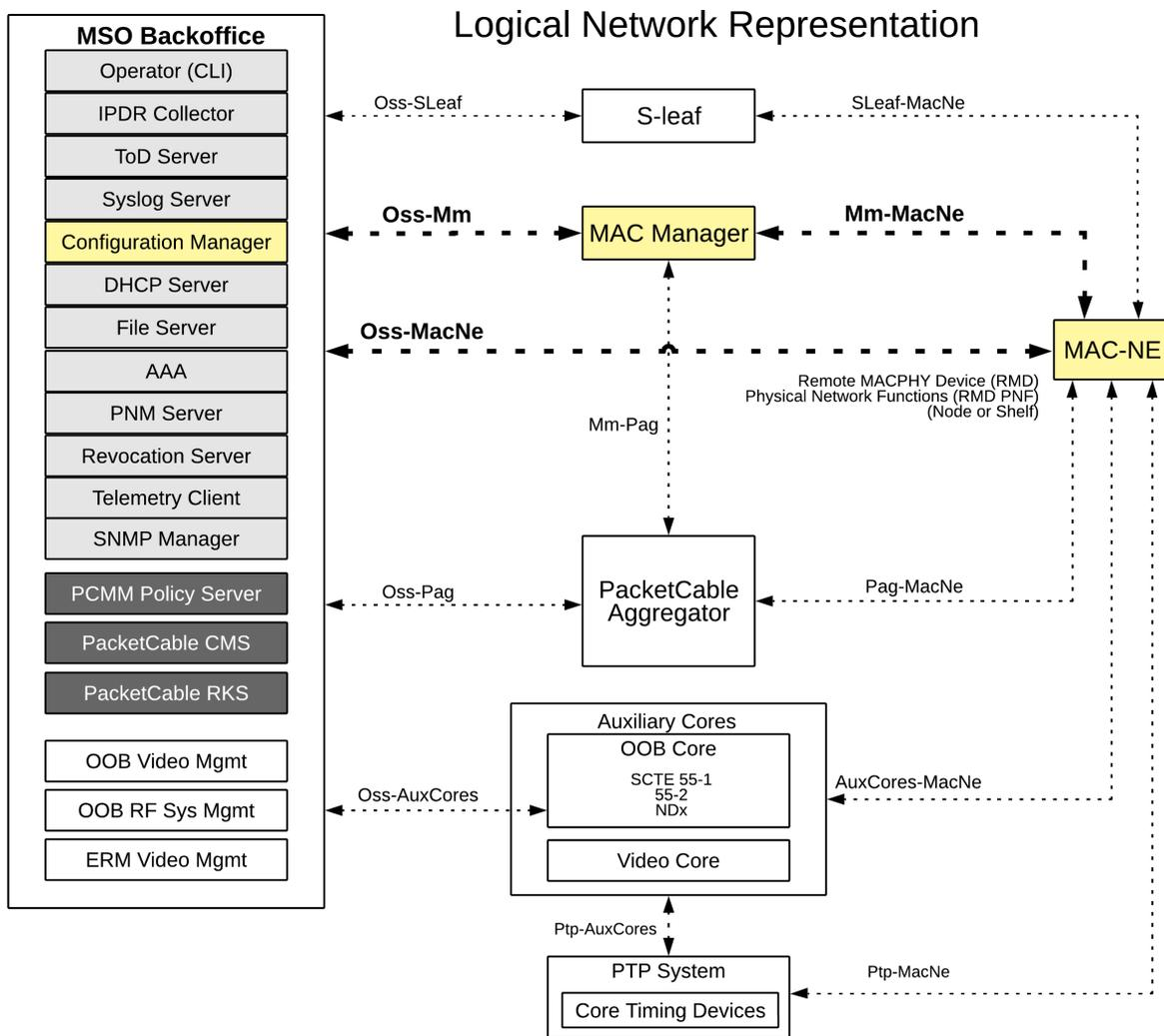
**Figure 2 - YANG-based Configuration Template Framework Scope**
