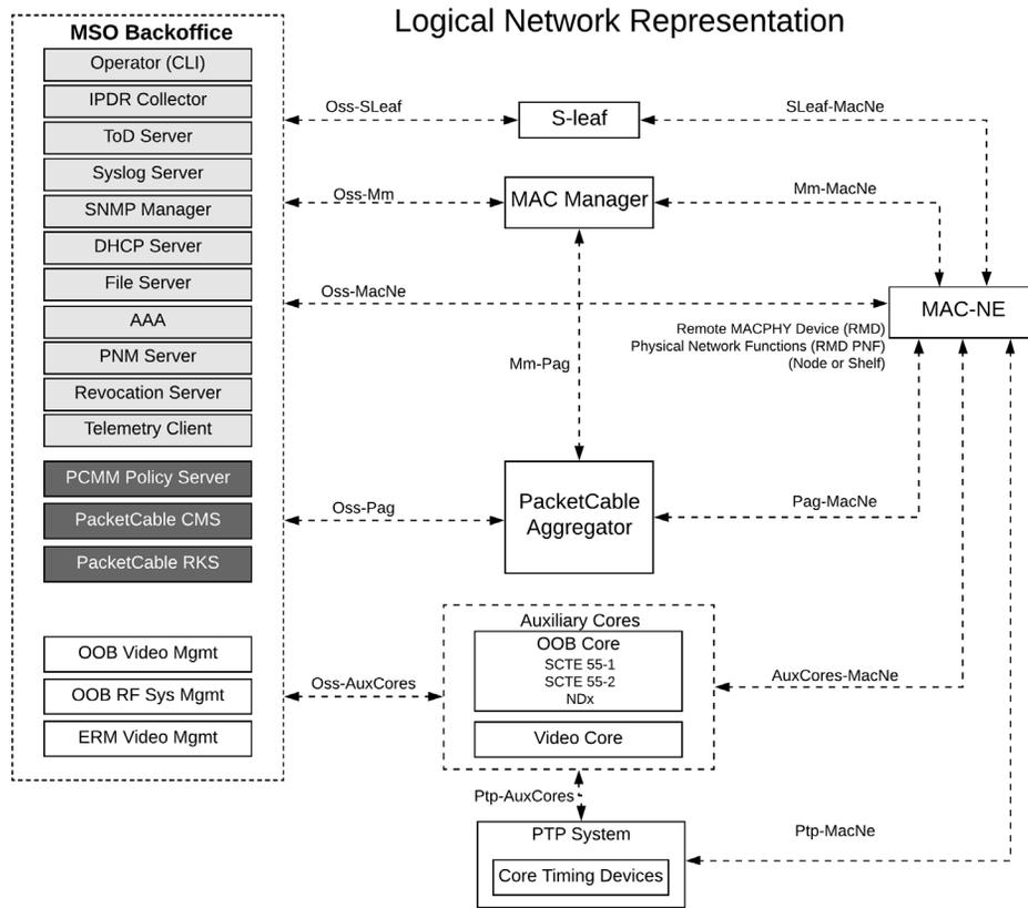
**Figure 1 - FMA Phase 1 Reference Architecture**
