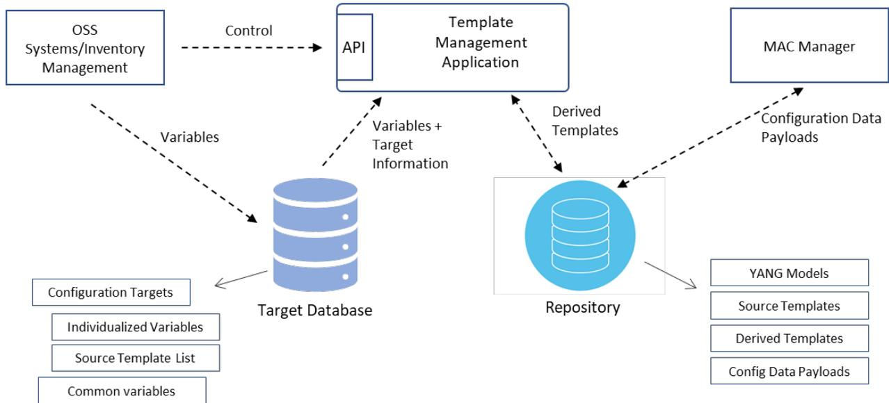
**Figure 6 – Template-Oriented Configuration Management System**
