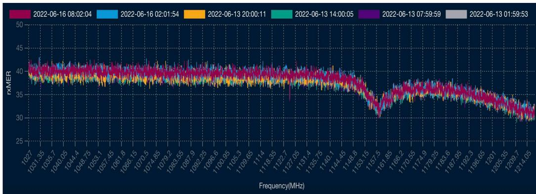
**Figure 8 – (Lab) Sample Cable Modem from Cluster A**
