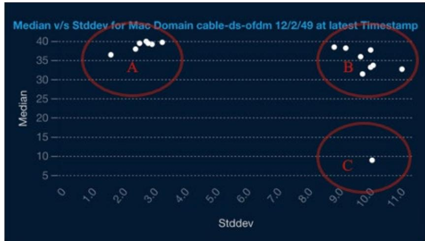
**Figure 7 – (Lab) 1.0-1.2 GHz Spectrum Med Var Plot**
