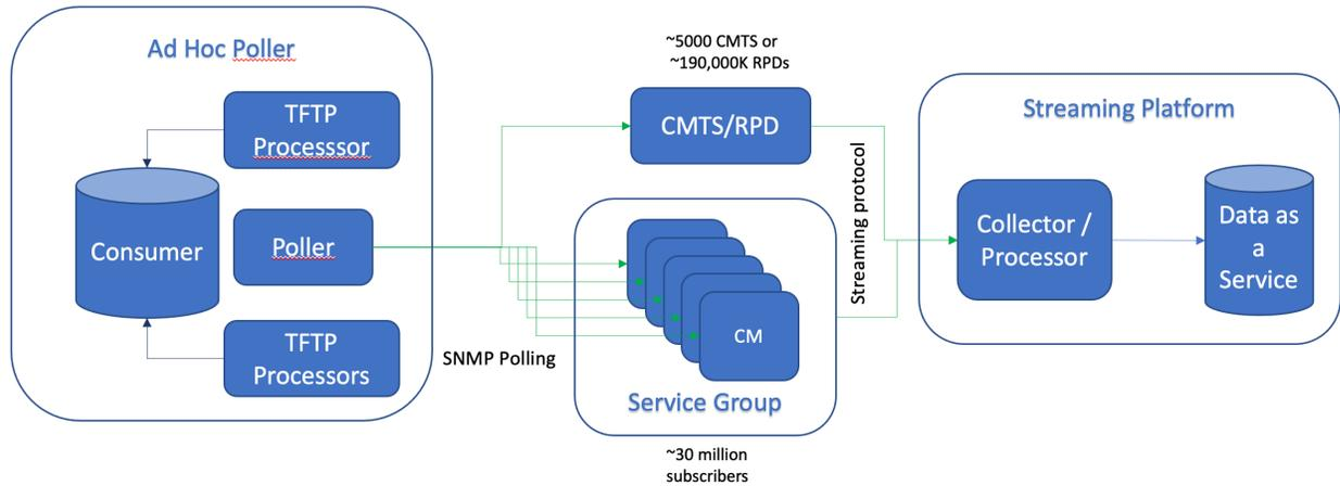
**Figure 6 – Modern Streaming Telemetry Data Architecture**
