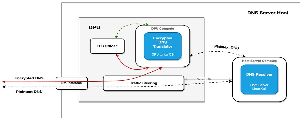
**Figure 6 – Encrypted DNS Using DPUs Block Diagram**
