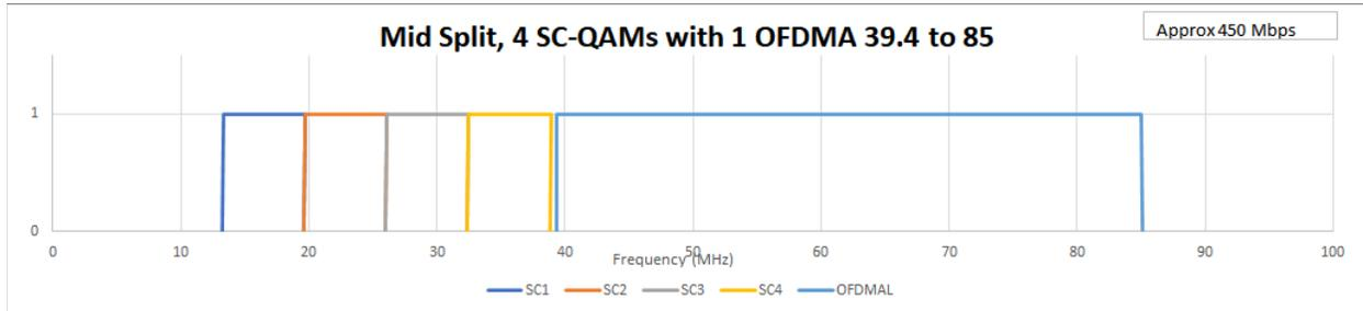
**Figure 12 – Mid-Split Channel Configuration of 4x SC-QAM + OFDMA**
