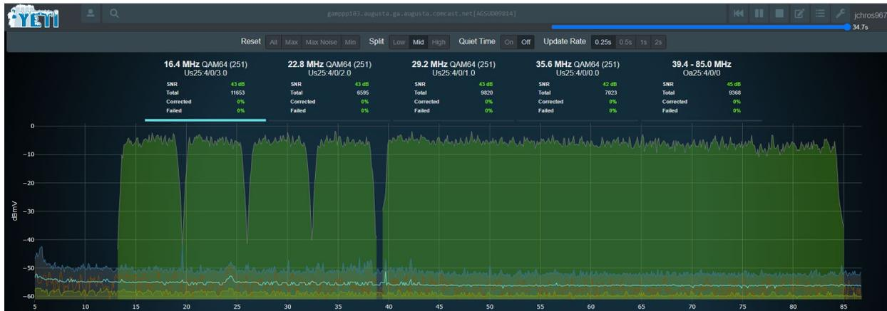
Figure 16 – Mid-Split Full Channel Configuration of SC-QAM + OFDMA
