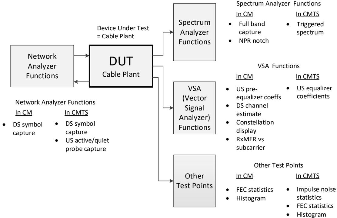
**Figure 1 - DOCSIS 3.1 "test points" for an HFC network.**
