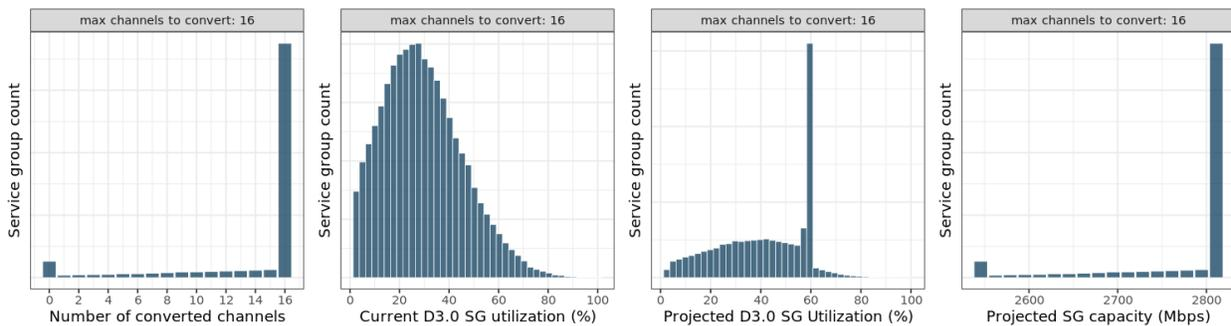
**Figure 5 - Analysis exploring converting up to 16 SC-QAM channels to OFDM. The number of converted channels is specific to each service group and selected such that projected D3.0 service group utilization does not exceed 60%.**
