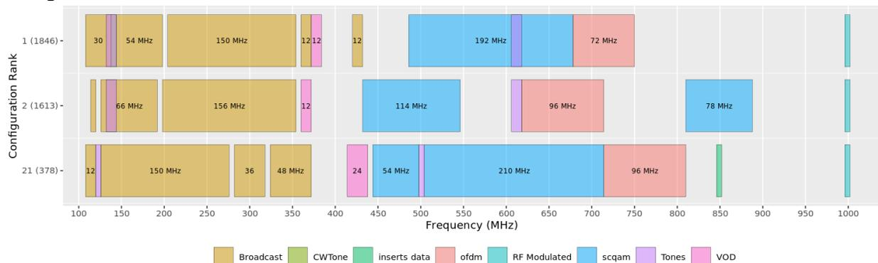
**Figure 6 - Example of three common downstream spectrum configurations.**
