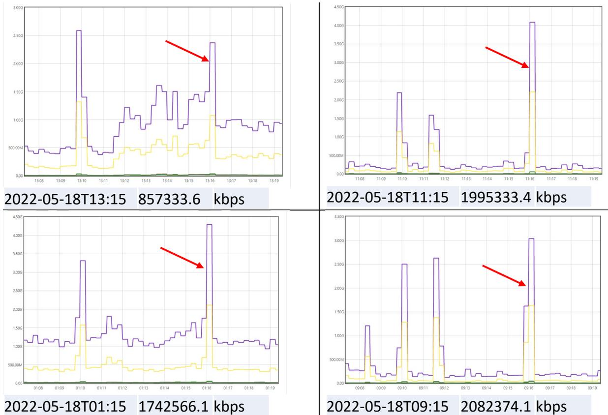
**Figure 10 - Speed test results for a 2 Gbps speed tier. There are no RF issues observed for this cable modem and corresponding node. However, utilization levels during the speed test have an impact on the results. Purple lines are total octets at service group level while yellow lines are total octets for the OFDM channel. The load telemetry data is displayed with a delay compared to speed test timing displayed in the bottom of each graph and indicated by a red arrow.**
