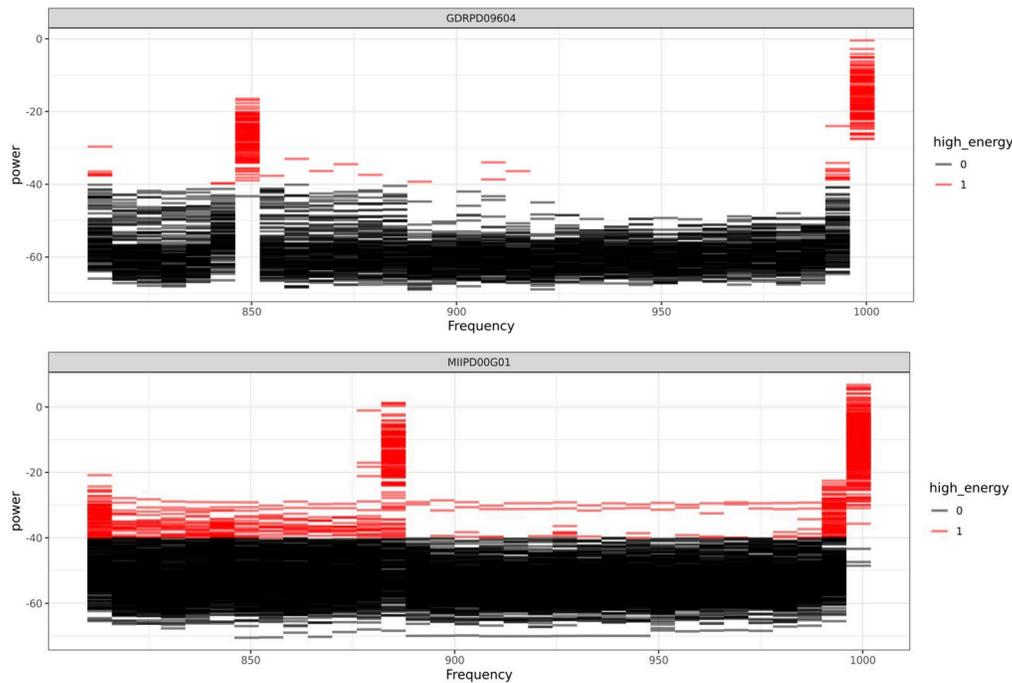
**Figure 8 - Example of two “conflicts” picked up by the vacancy detection algorithm: (1) a local insert was confirmed at 850 MHz, and (2) ingress due to police repeater was picked up at 885 MHz on a different RPD.**
