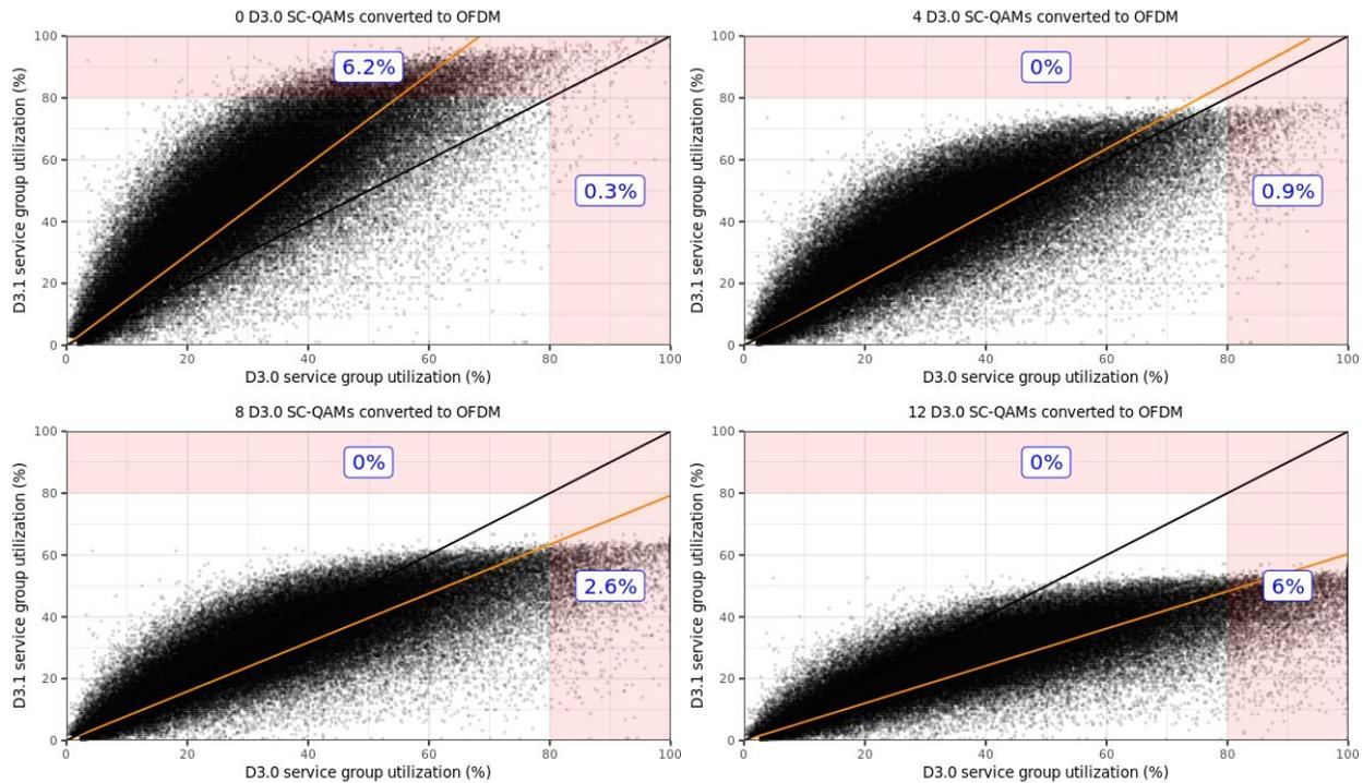
**Figure 4 - Joint D3.0 and OFDM distributions at different number of SC-QAM channels converted to OFDM. (Top left) 0 channels converted—representing the baseline, (top right) 4 channels converted, (bottom left) 8 channels converted, and (bottom right) 12 channels converted.**
