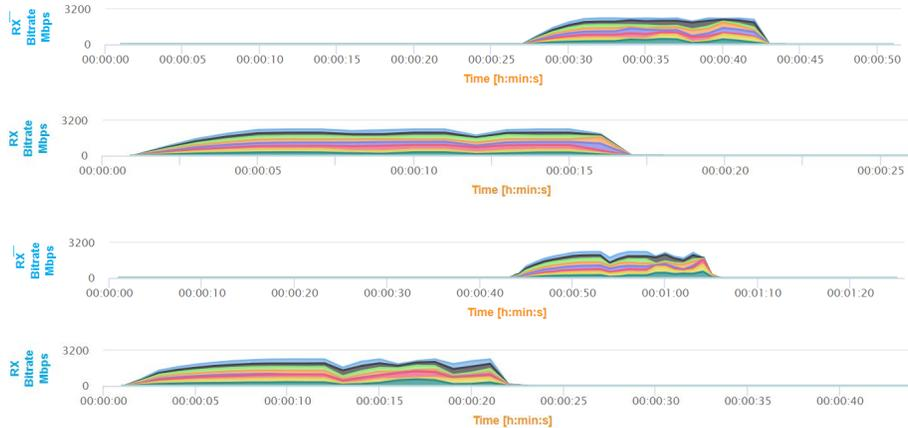
**Figure 9 - The data throughput over iCMTS (top 2 panels) and vCMTS (bottom 2 panels) for a single D3.1 cable modem demonstrating speeds in the 2.3-2.4 Gbps range. The different colors indicate different TCP flows utilized by the speed test.**
