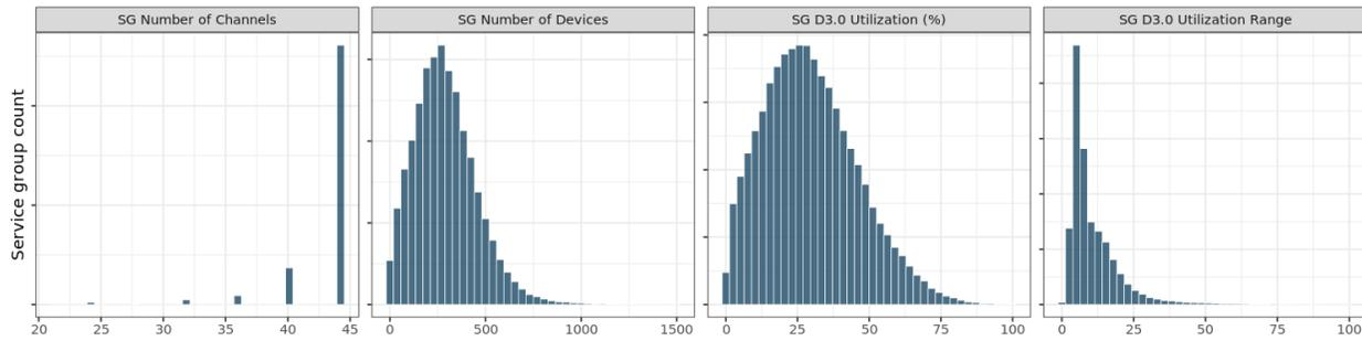
**Figure 2 - Distributions of (1) number of D3.0 channels per service group, (2) number of devices per service group, (3) D3.0 service group utilization, and (4) D3.0 utilization range across channels within the service group.**
