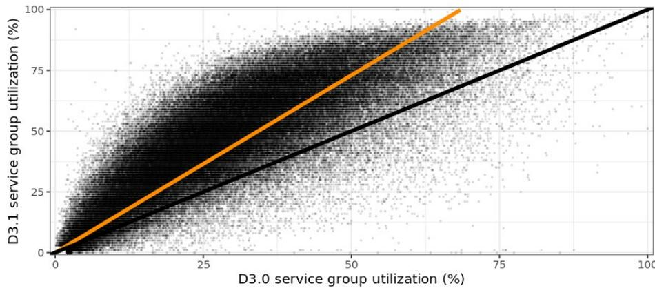
**Figure 3 - Joint D3.0 and OFDM distribution shown as a scatter plot. The black line is the bisector (45 deg. angle) and the orange line is line-of-best-fit for the scatter.**
