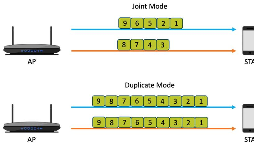
**Figure 14 – Multi-Link Joint Mode**
