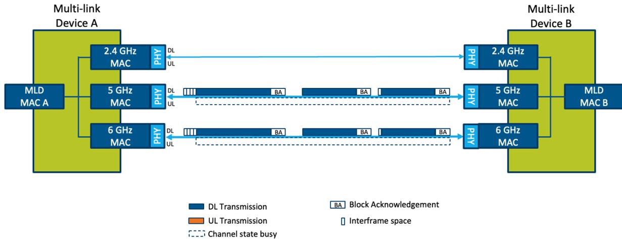
**Figure 6 – Synchronous Multi-Link Channel Access**
