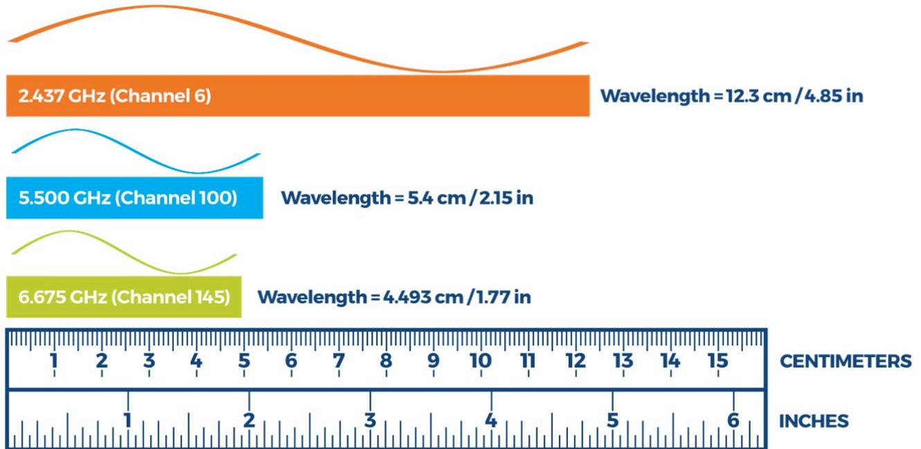
**Figure 20 – Wavelength of 2.4, 5, and 6 GHz**
