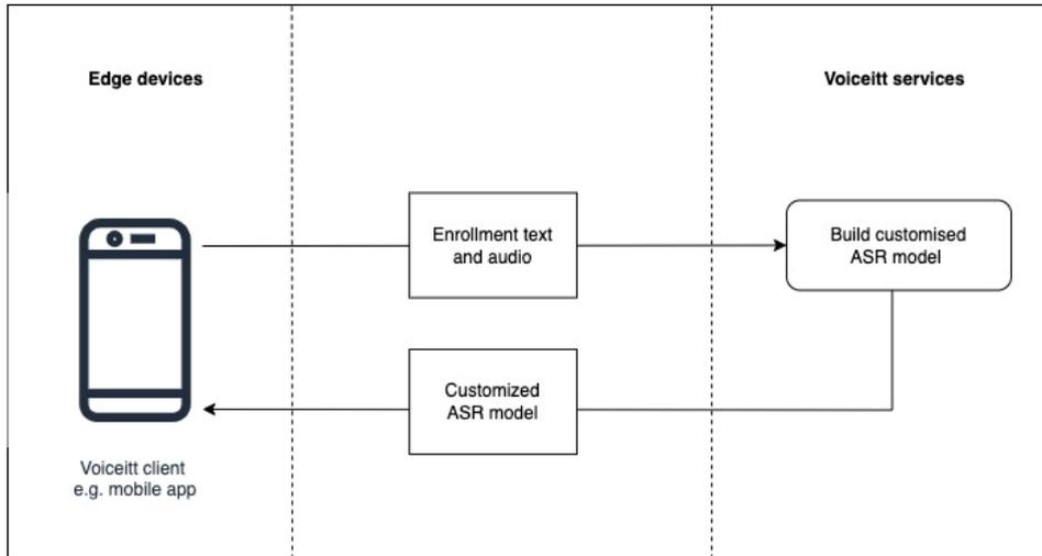
**Figure 1 – customized model downloaded onto the edge device**
