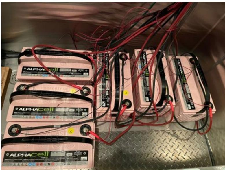
**Figure 5 – Tested Batteries for Temperature Effect**
