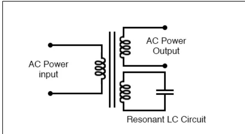
**Figure 4 - Simple circuit diagram of a ferroresonant transformer**
