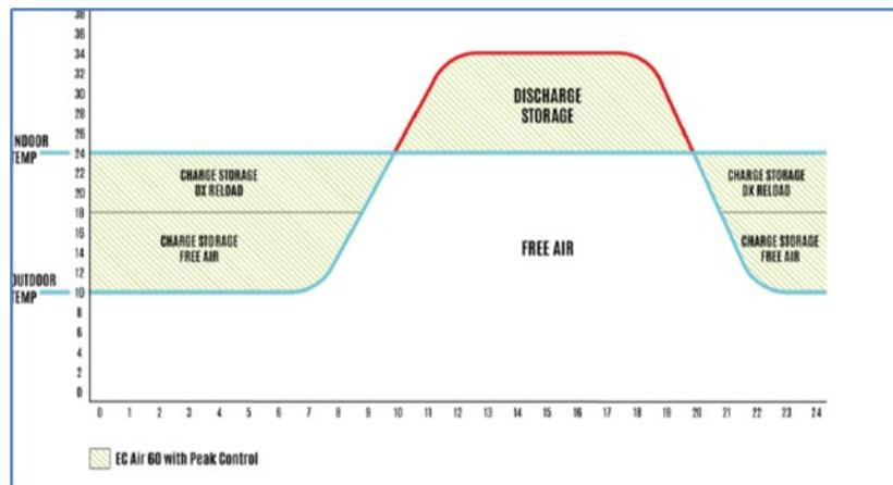
**Figure 9 - Phase Change Material and Free Air Cooling (Diagram Courtesy of Energy Cool<sup>®</sup>)**
