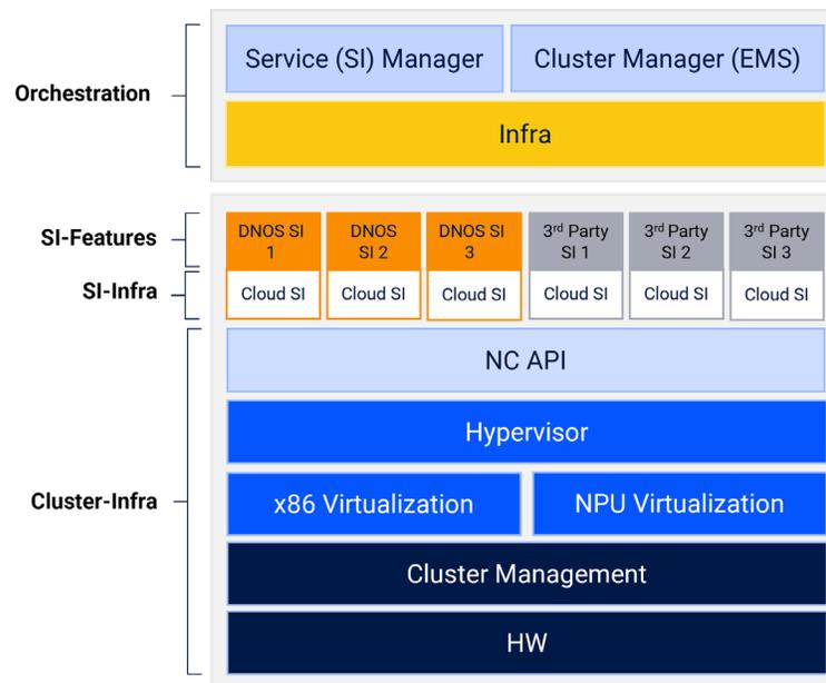
**Figure 14 - Software Architecture of the Network Cloud**
