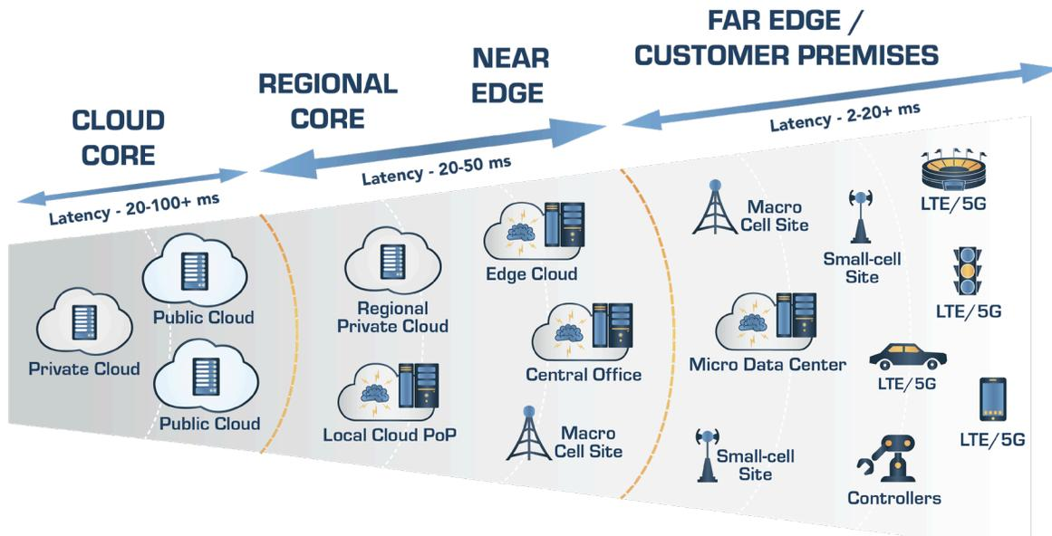
**Figure 6 - Components of the Edge Cloud**
