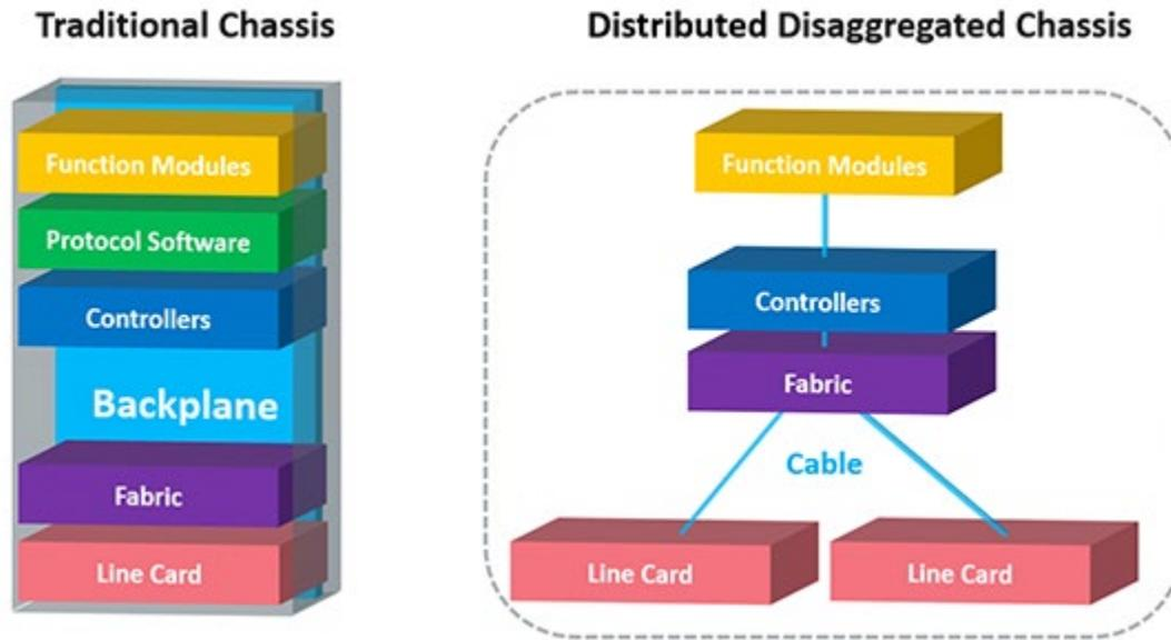
**Figure 9 - DDC/DDBR Architecture**
