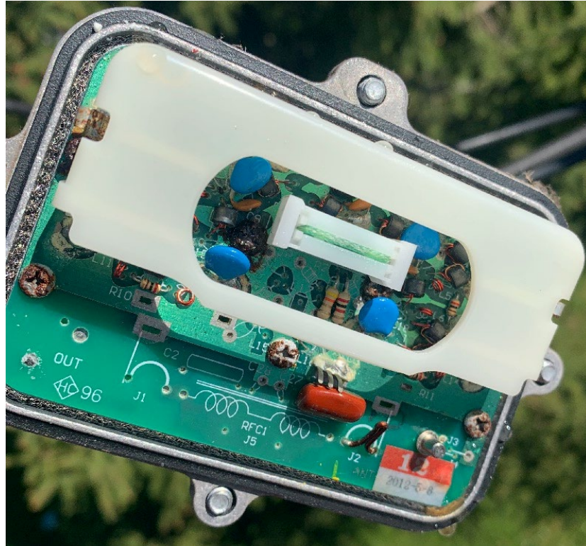
Figure 4 - Water-soaked tap faceplate, water droplets visible (Courtesy of James Medlock, Akleza)
