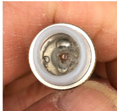
Figure 10 - Water visible after vacuum is applied
