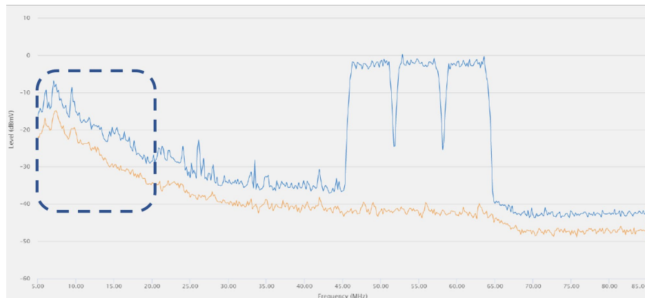
Figure 3 – Noisy Spectrum Below 20 MHz
