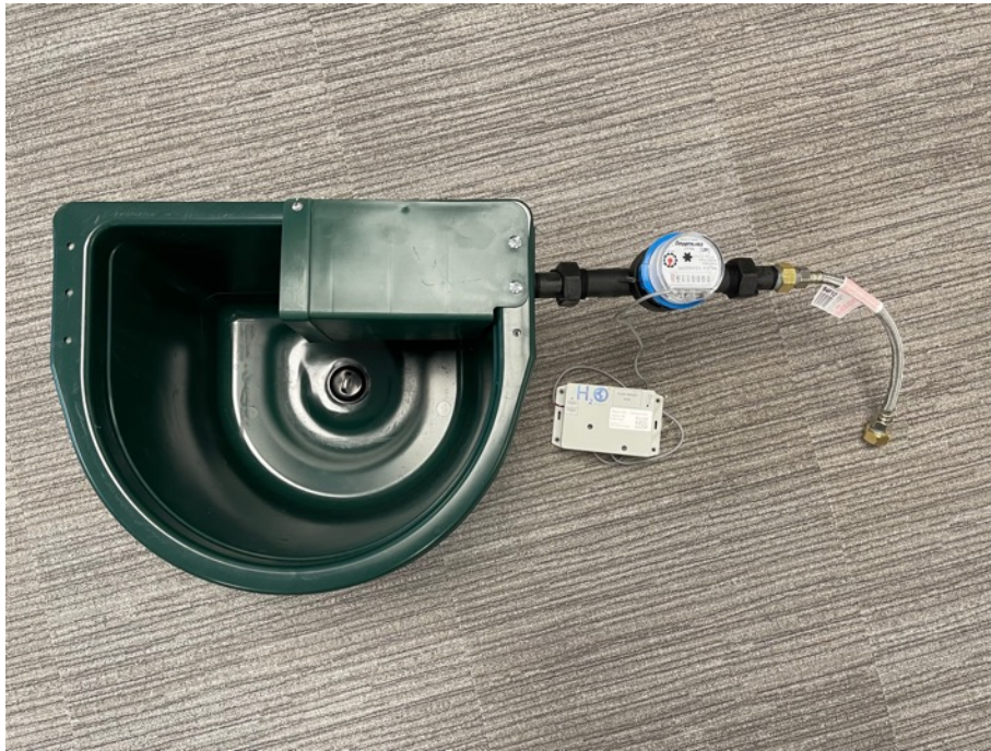
Figure 7 - Water meter and LoRa pulse sensor solution
