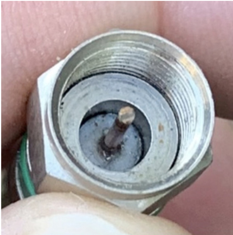
Figure 1 - F-connector not flush with the cable's dielectric
