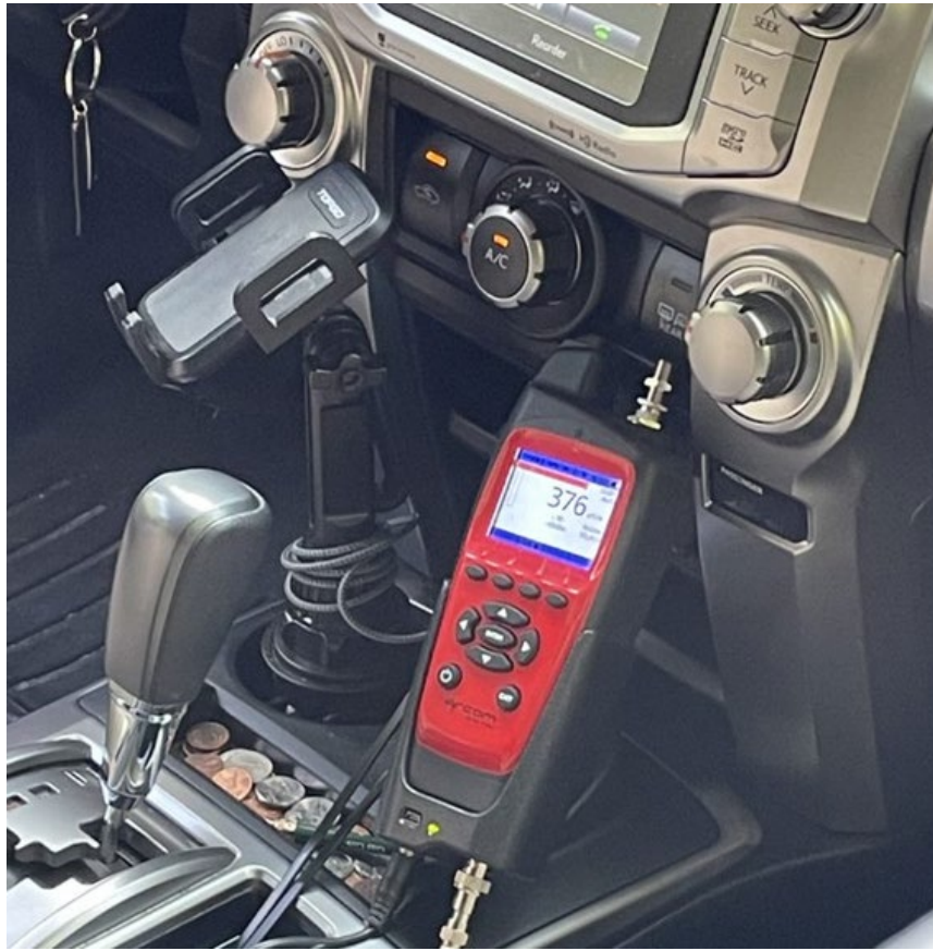
Figure 12 – Leakage Detection in a Stationary Vehicle
