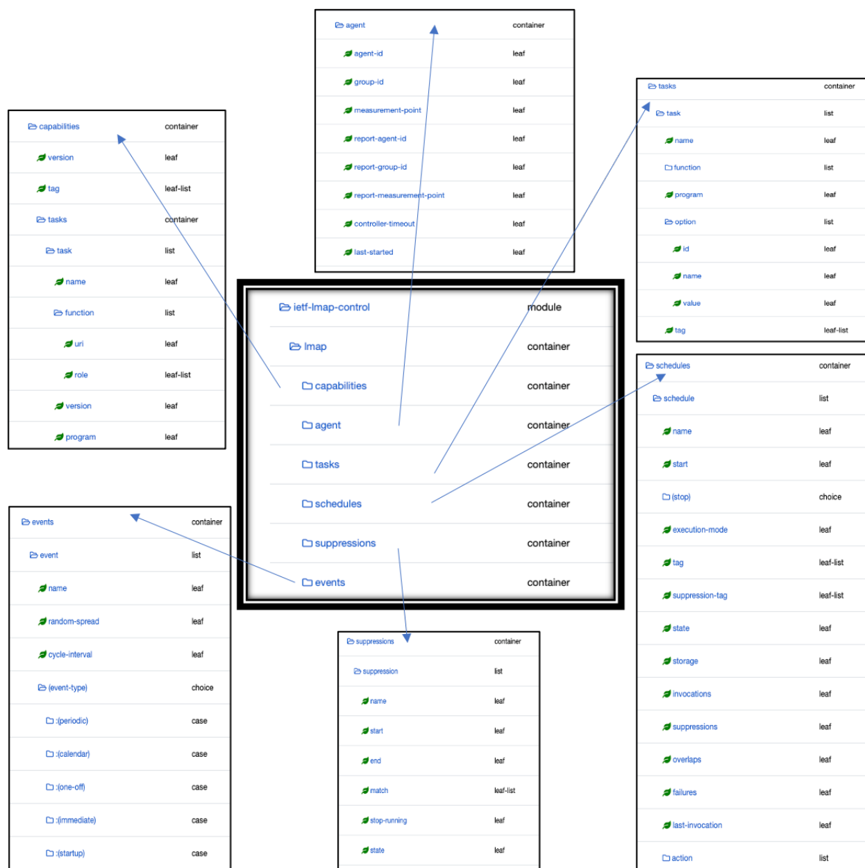
Figure 7 – High level view of the LMAP-Control YANG model
