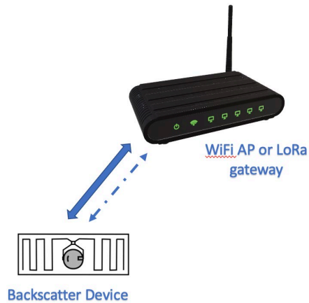
Figure 11 - Backscatter using Wi-Fi or LoRa signals
