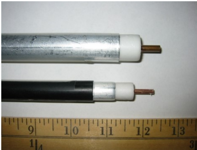
Figure 43 - Examples of hardline coaxial cable: unjacketed 0.750 inch diameter (top) and jacketed 0.500 inch diameter (bottom)
