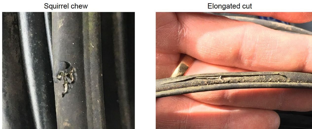
Figure 11 - Rodent chew compared to elongated cut, common coaxial damages (Courtesy of Skip Palinkas, PPC)
