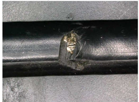
Figure 8 - Coaxial jacket breach near tap-side connector
