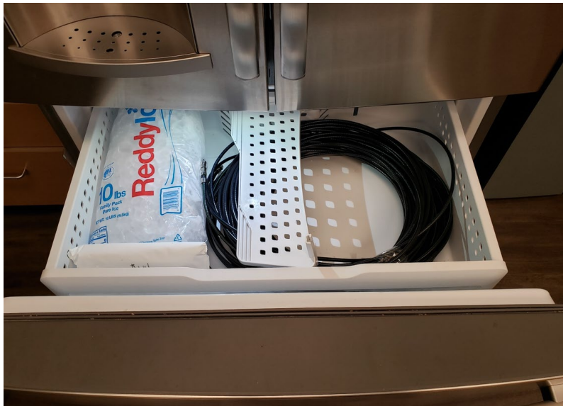
Figure 14 - Freezing the water-soaked drop cable
