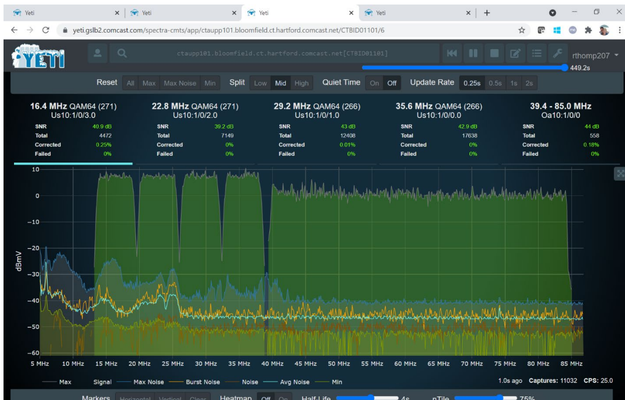
Figure 5 – Activated Mid-Split of 4xSC-QAM + OFDMA
