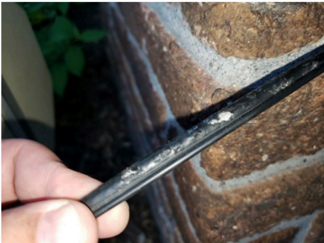
Figure 19 - Damaged coax jacket where water was able to enter the cable
