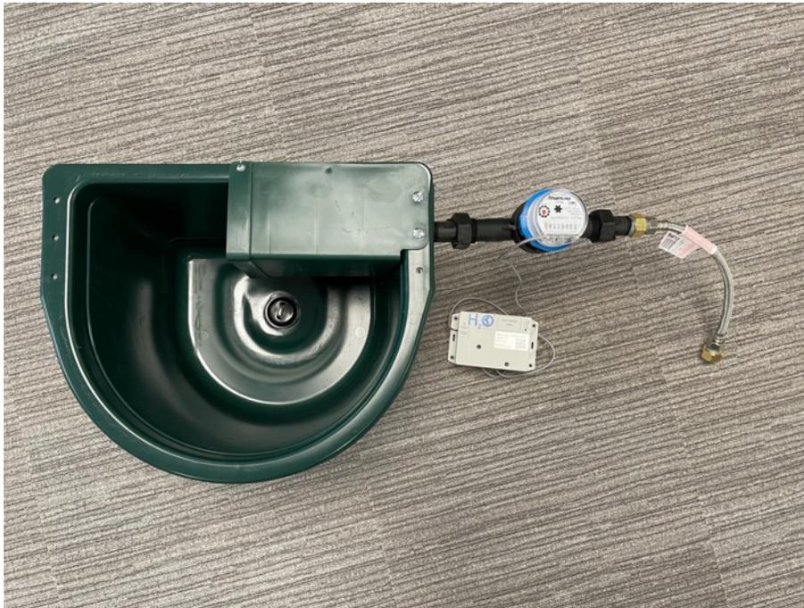
**Figure 7 - Water meter and LoRa pulse sensor solution**
