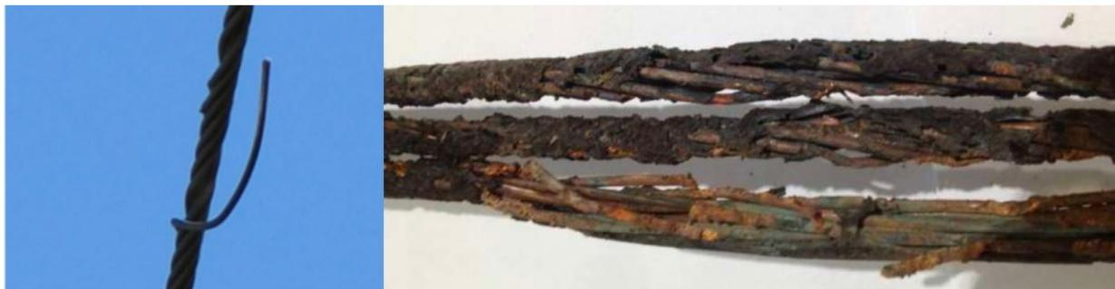
**Figure 10 – Examples of failing in-service conductors**
