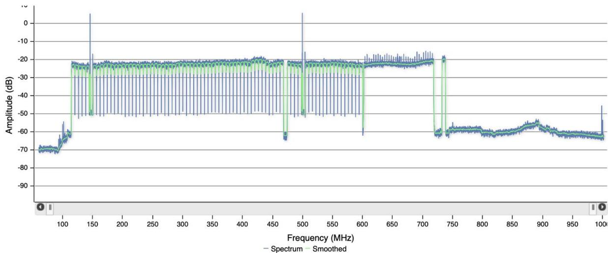
**Figure 6 - Flat frequency response after faceplate replacement**
