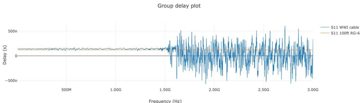
**Figure 30 - Group delay plot of  $S_{11}$  values for a water-soaked cable (WWI cable) and a clean, unimpaired, dry cable, both 100 feet of Series 6 cable**
