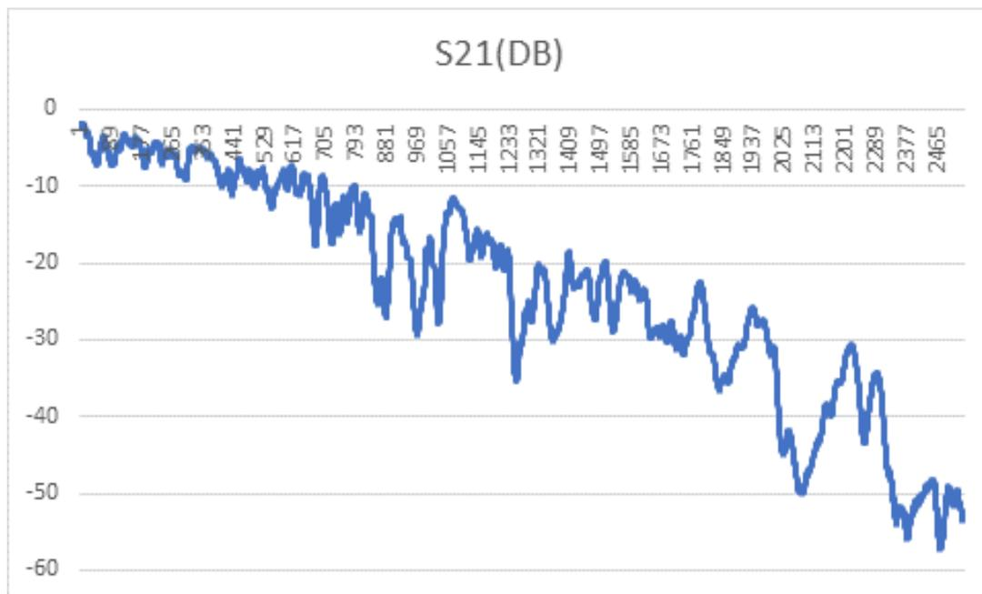
**Figure 27 - S<sub>21</sub> for a water-soaked drop**
