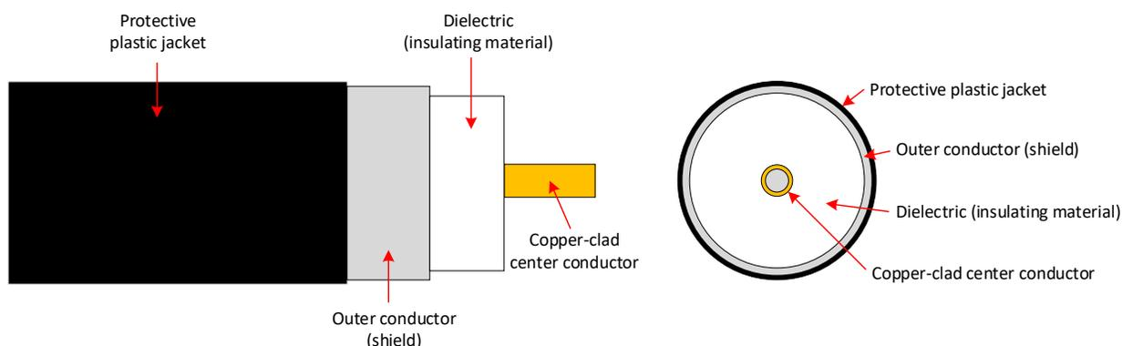
**Figure 42 - Coaxial cable side view (left) and end view cross-section (right)**
