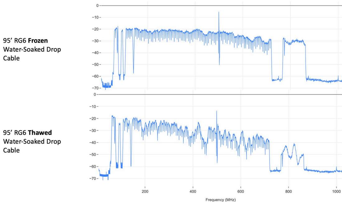
Figure 15 - Frozen (top) compared to thawed (bottom) frequency response
