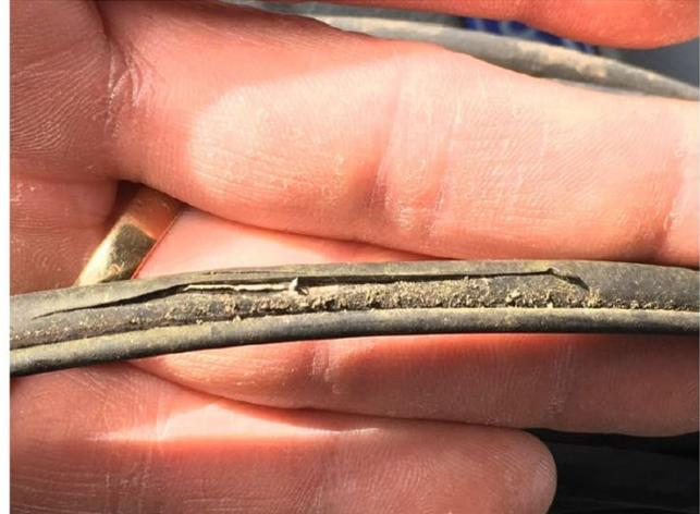
**Figure 11 - Rodent chew compared to elongated cut, common coaxial damages**
