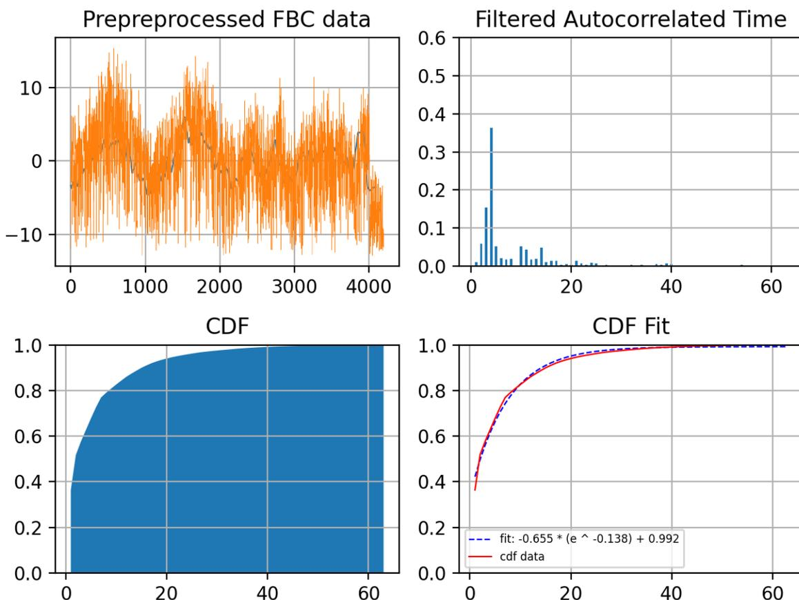
**Figure 33 - A confirmed wet drop from the field which has been installed in the PNM lab at CableLabs, and the CM on the end of the drop used to gather spectrum data then processed with the CDF curve fitting method**
