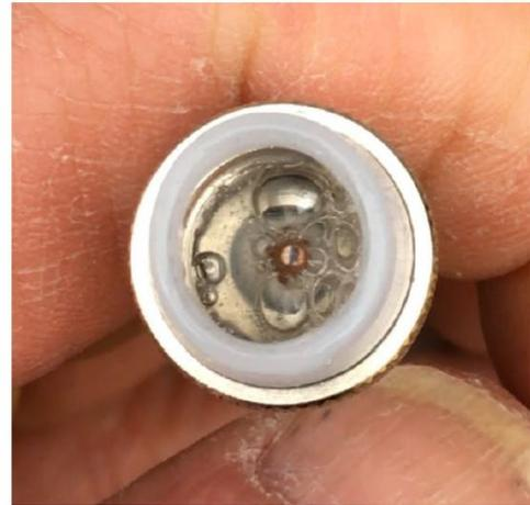
**Figure 10 - Water visible after vacuum is applied**
