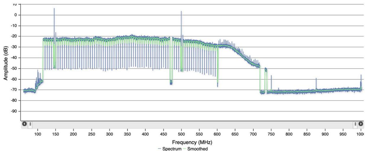
**Figure 5 - Roll-off frequency response of water damaged tap port**
