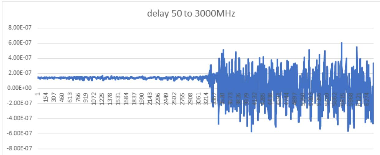
Figure 28 - Group delay for a water-soaked cable
