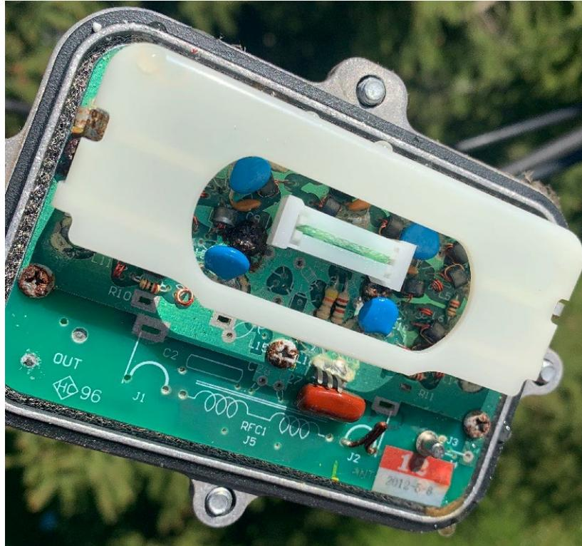
**Figure 4 - Water-soaked tap faceplate, water droplets visible**
