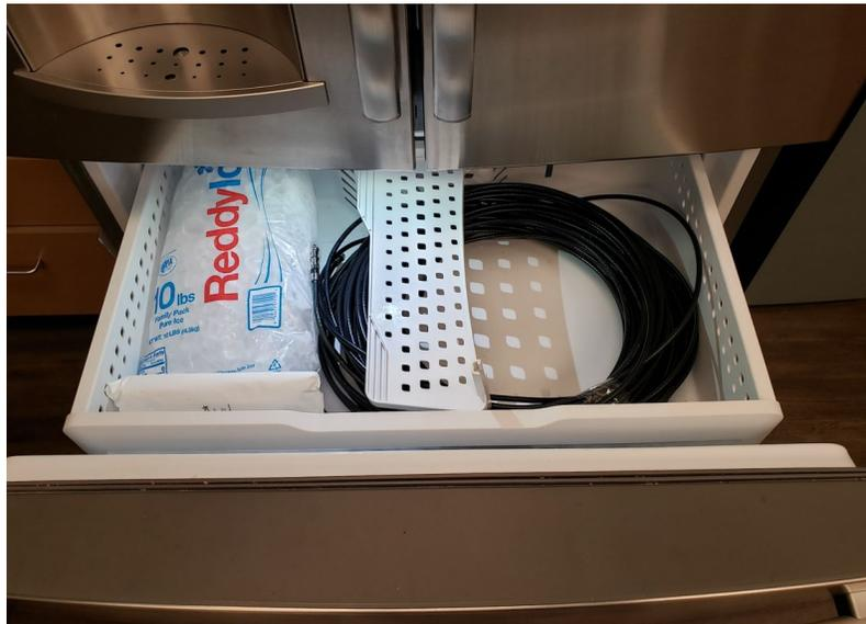
**Figure 14 - Freezing the water-soaked drop cable**
