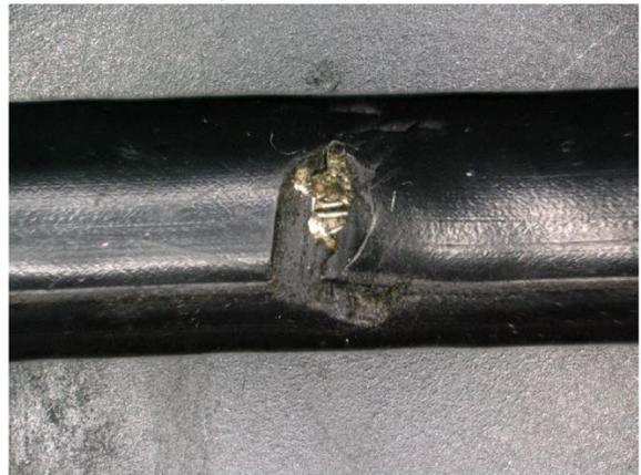
**Figure 8 - Coaxial jacket breach near tap-side connector**
