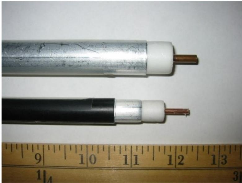
**Figure 43 - Examples of hardline coaxial cable: unjacketed 0.750 inch diameter (top) and jacketed 0.500 inch diameter (bottom)**
