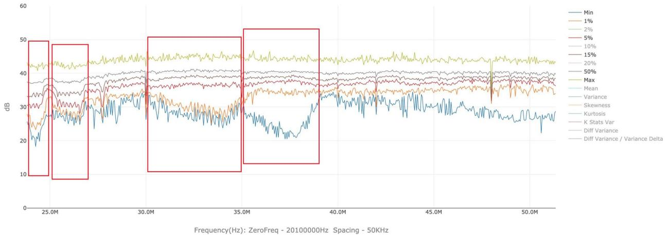
**Figure 7 – Percentiles and min, max values calculated for each subcarrier**
