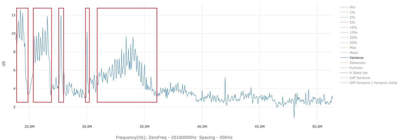
**Figure 8 – Variance values calculated for each subcarrier**
