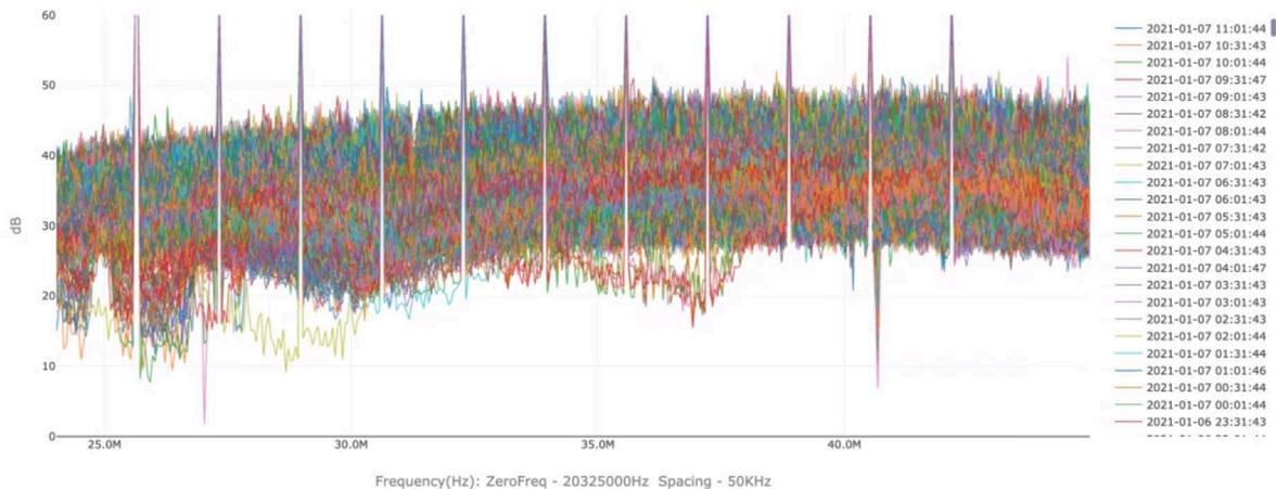
Figure 4 – Multiple US RxMER samples, OFDMA channel, Single CM (field)
