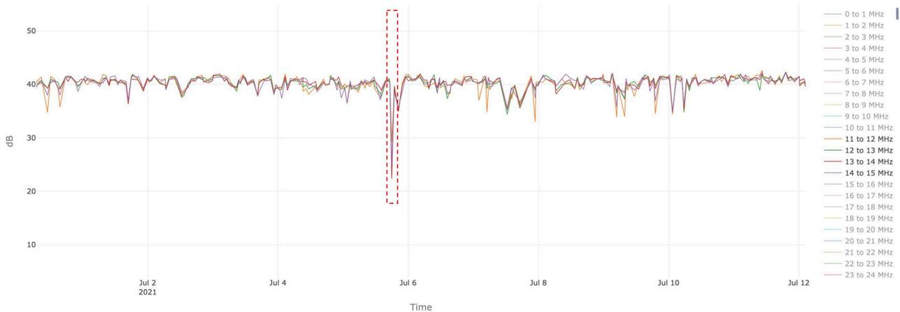
**Figure 16 – Intermittent issue observed on RxMER time series**
