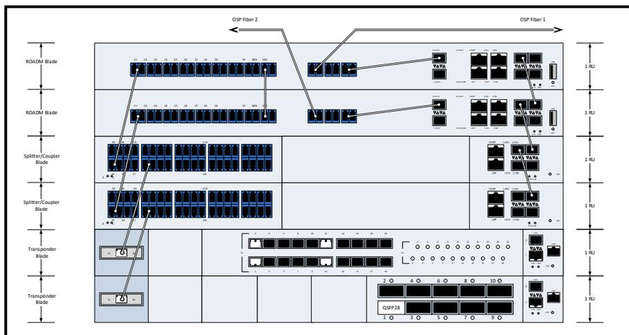
**Figure 4 – ROADM Blades, Splitter/Coupler Blades, and Transponder Blades**
