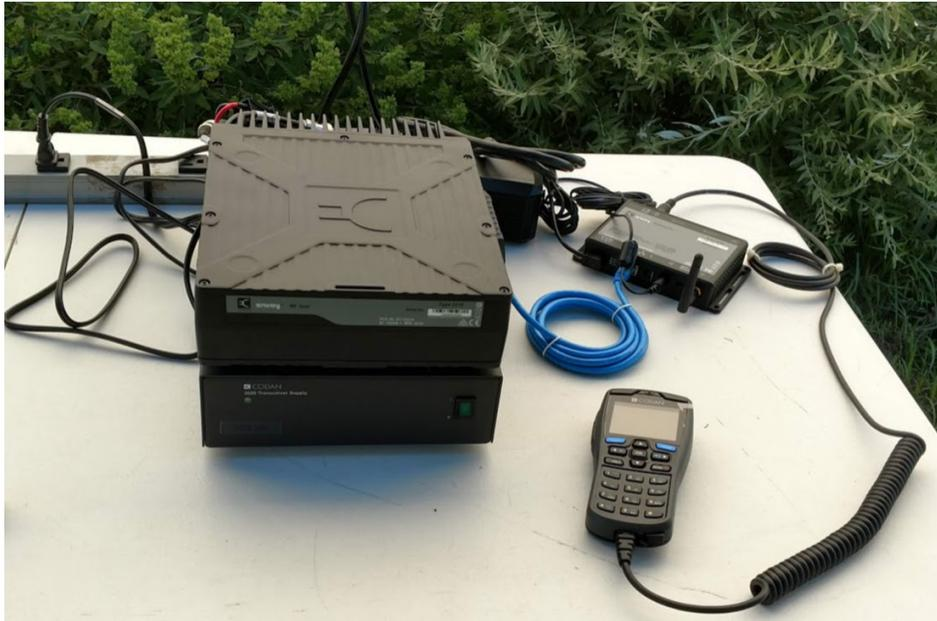
**Figure 5 - SCTE Portable Radio and Power Supply**
