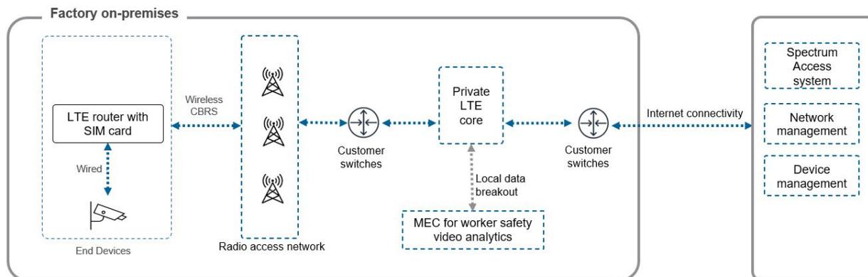
**Figure 7 - Deployment architecture**
