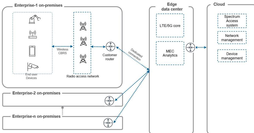
**Figure 3 - Network core at edge data center**
