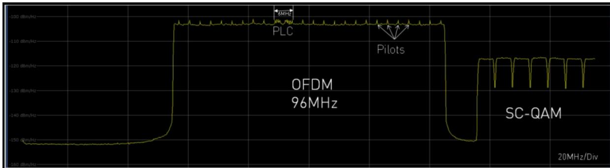
**Figure 5 - Example OFDM channel highlighting the PLC [2].**
