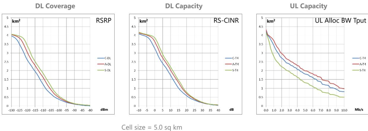
**Figure 6 – One-mile cell radius suburban scenario - 45' Height Antenna**
