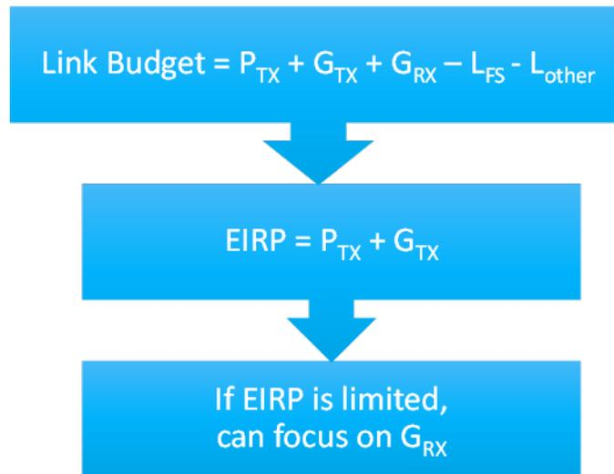
**Figure 3 – Link budget vs EIRP**
