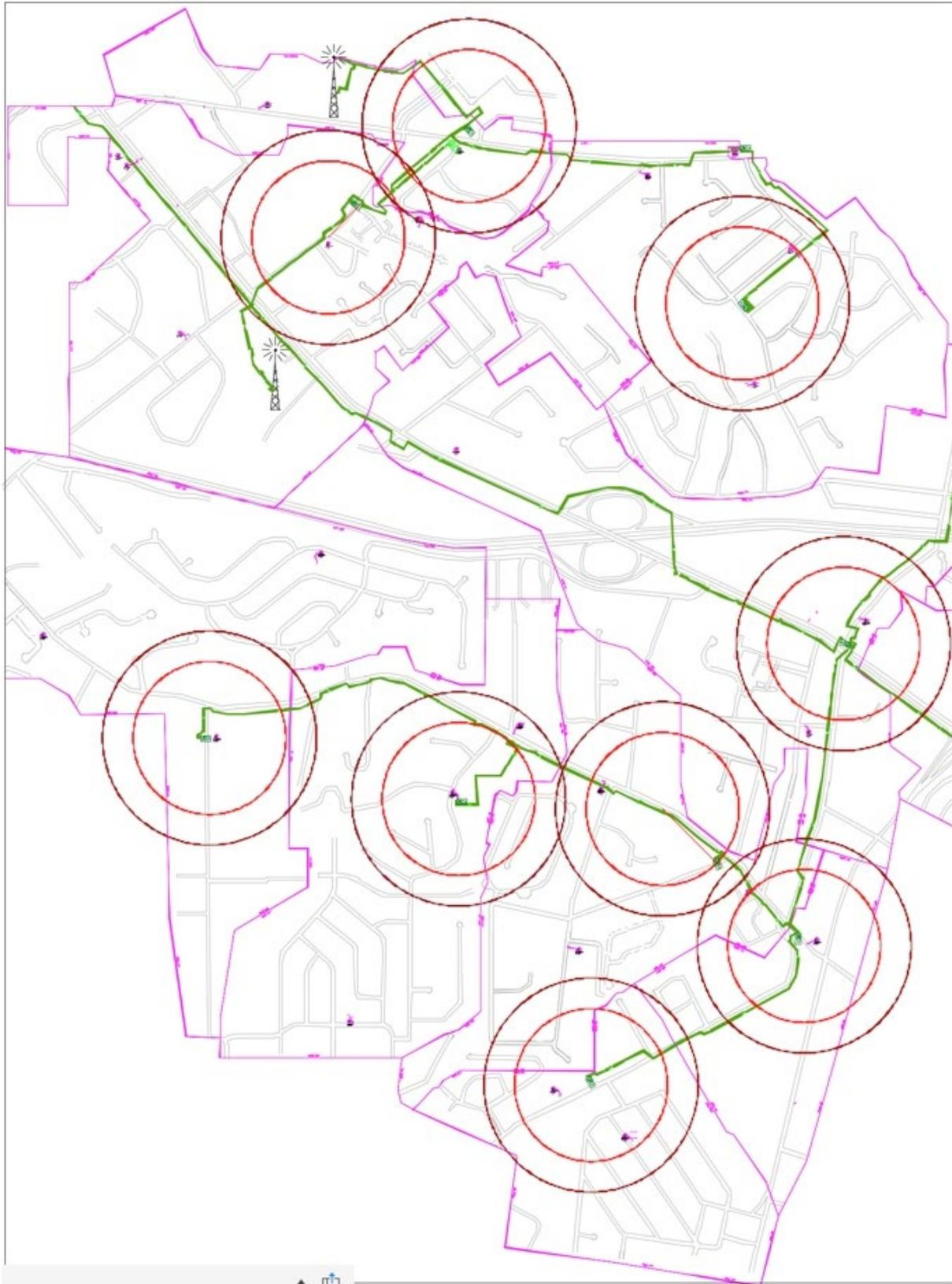
**Figure 23 – N+6 Suburban area with Small cells at Fiber Node**
