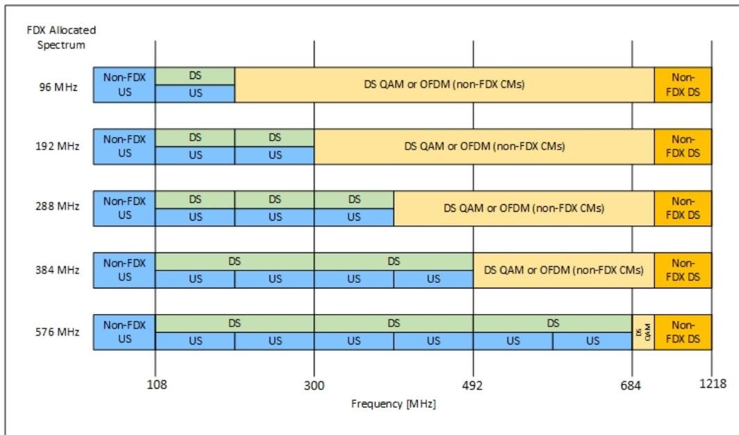
Figure 13 – Full Duplex DOCSIS (FDX) Spectrum Band Options
