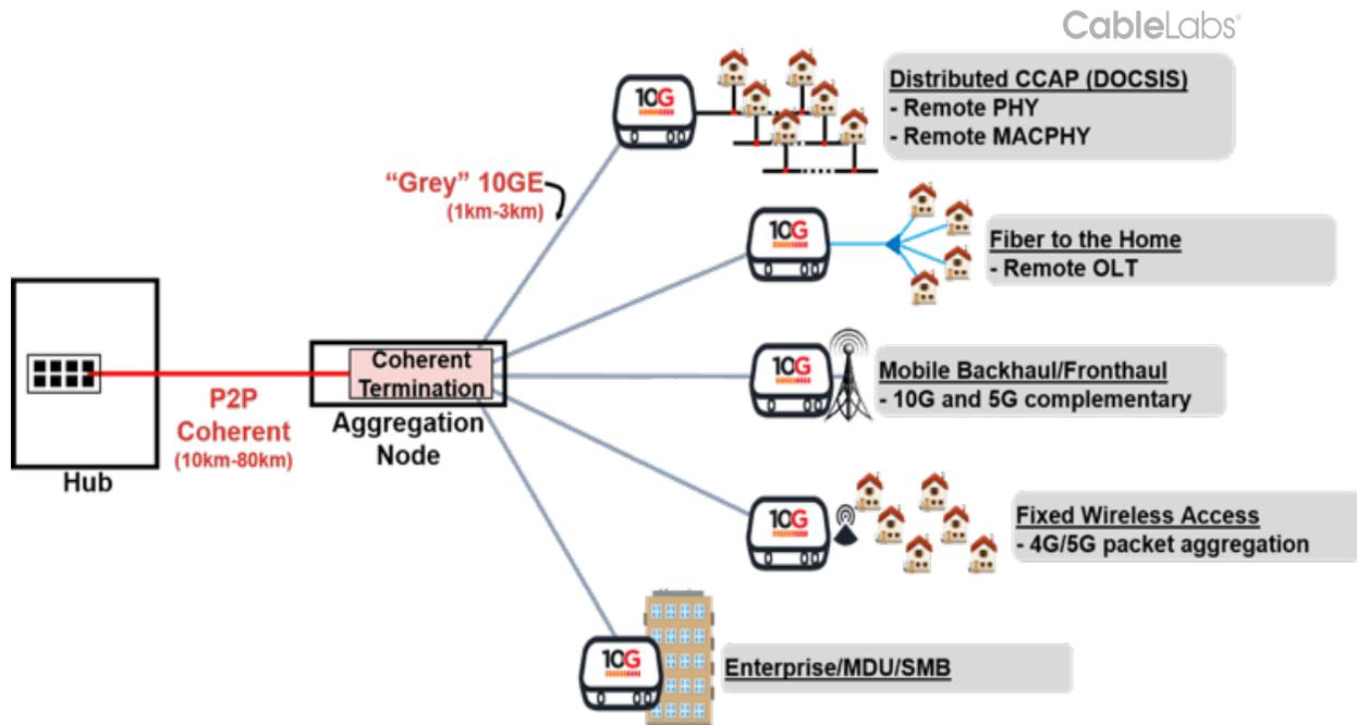
Figure 12 – 10G™ Converged Optical Network – Distributed Access Architecture vision
