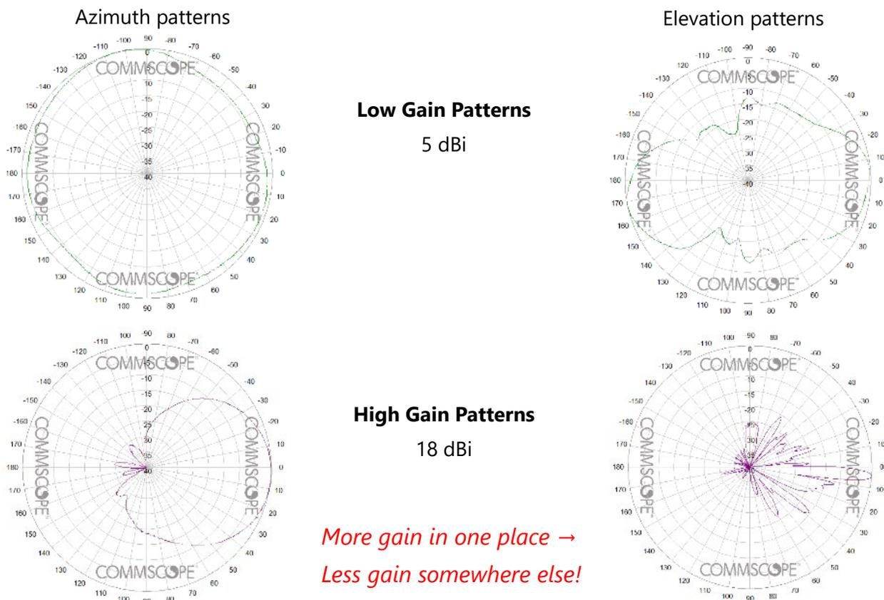
**Figure 4 – Antenna Gain**
