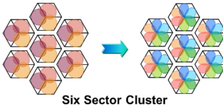
**Figure 2 – Sector antennas – Three to Six Sectors**
