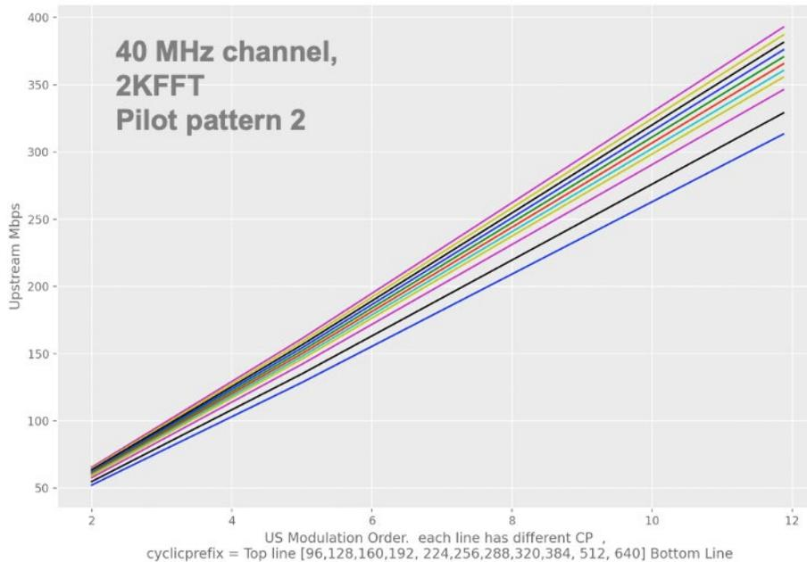
**Figure 9 – OFDMA capacity change for different CP**
