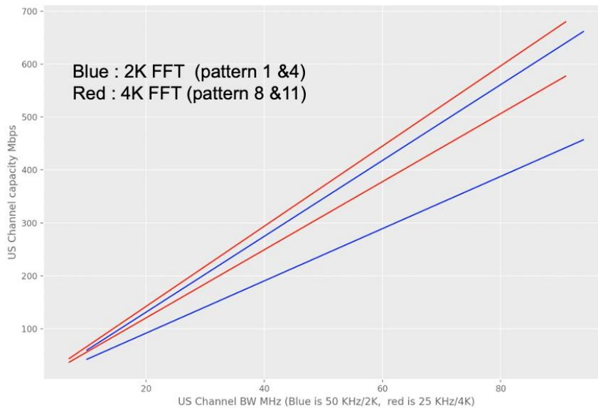
**Figure 11 – OFDMA capacity change 2K vs 4K FFT**
