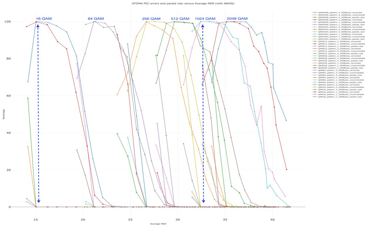
Figure 6 – OFDMA FEC Performance (200 byte packets)
