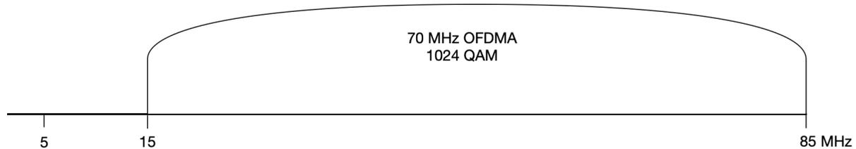
Figure 32 – Mid-split with All OFDMA channel
