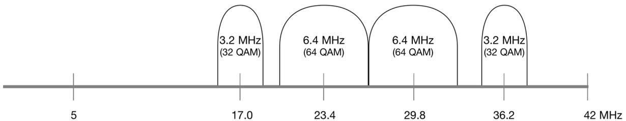
Figure 26 – Increasing Channel Width To Increase Upstream Capacity
