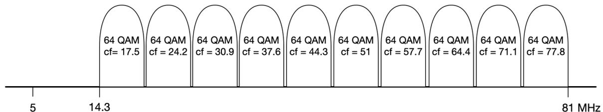
**Figure 30 – Mid-split with 10 SC-QAM channels**
