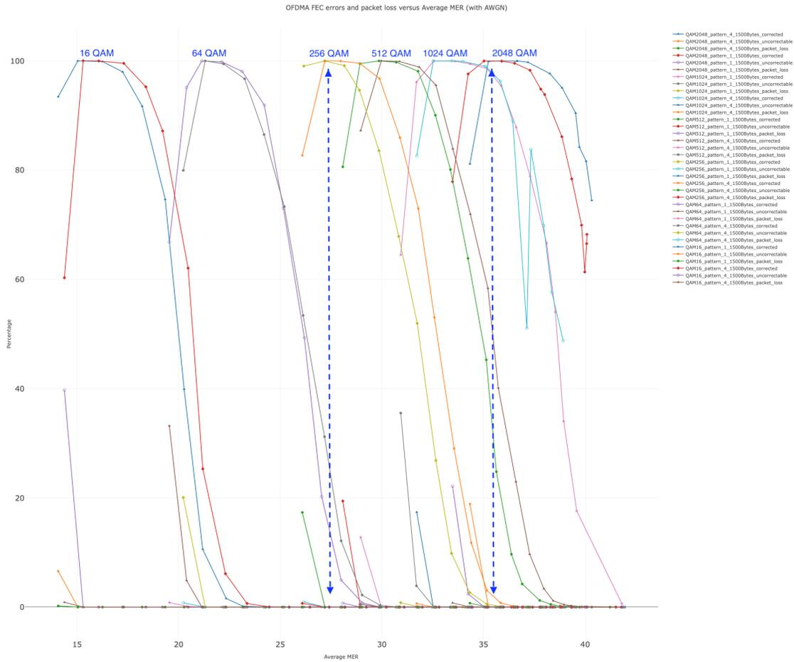
Figure 7 – OFDMA FEC Performance (1500 byte packets)
