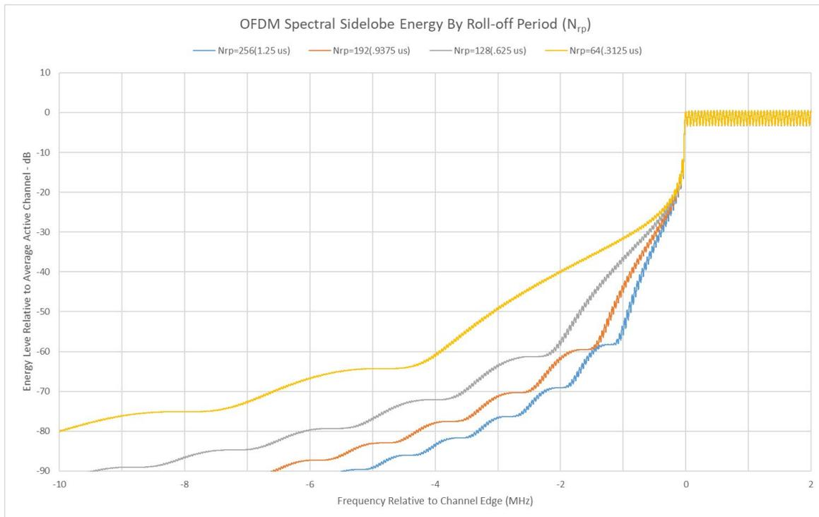
**Figure 15 – OFDM/A Spectral Sidelobes (impact on Adj. SC-QAM)**
