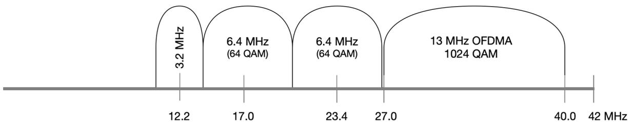
**Figure 29 – Sub-split HFC Network with OFDMA Channel**
