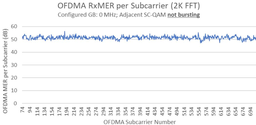
**Figure 19 – OFDMA RxMER (OFDMA bursting alone)**
