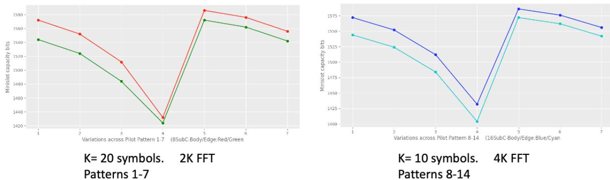
Figure 12 – OFDMA Minislot capacity change w Pilot Patterns
