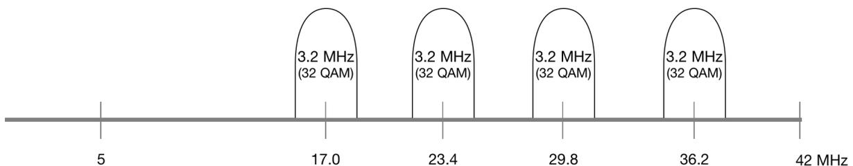
**Figure 25 – Large Guard Bands Between Upstream Channels**
