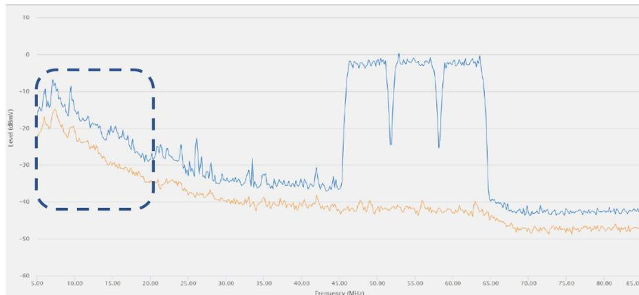
**Figure 3 – Noisy Spectrum Below 20 MHz**
