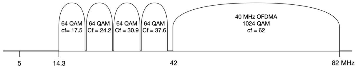
**Figure 31 – Mid-split with Both SC-QAM and OFDMA channels**
