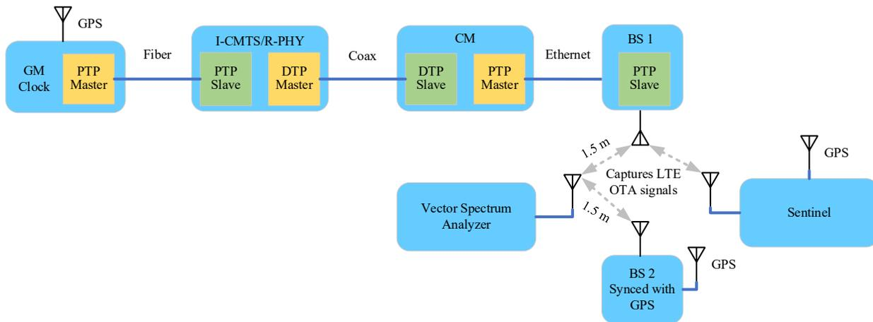
**Figure 3 - Block Diagram of LTE OTA Setup**
