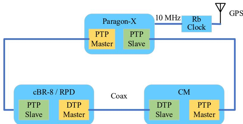
**Figure 2 - Block Diagram of DTP Performance Test Setup [9]**
