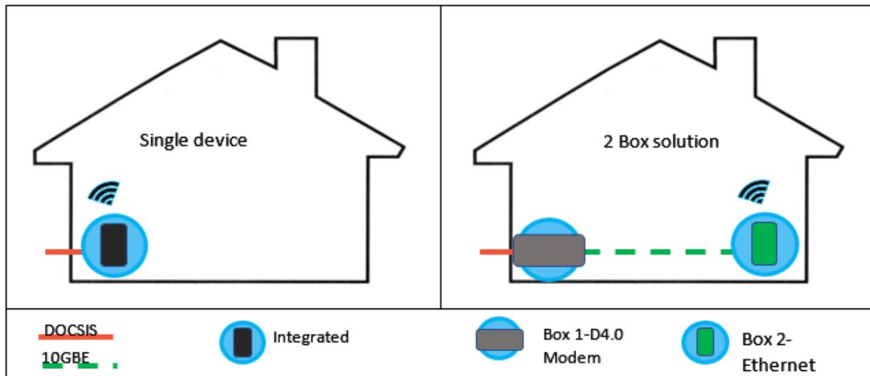
**Figure 19 - DOCSIS 4.0 CPE 1-Box vs 2-Box Installation**
