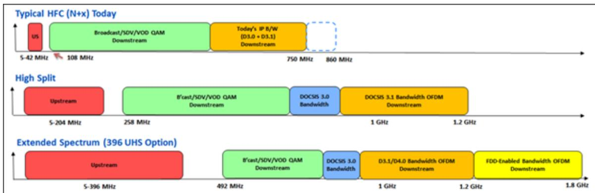
Figure 12 - Typical HFC vs High Split vs DOCSIS 4.0 Extended Spectrum
