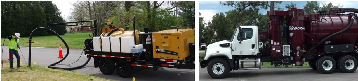
**Figure 7 - Examples of Vacuum Excavators<sup>2</sup>**
